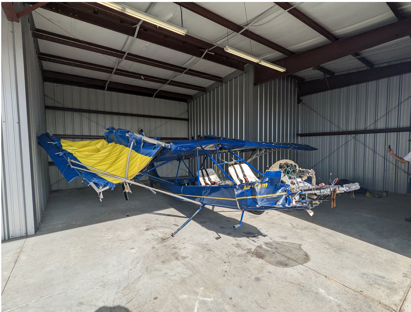
Photo 2 - Digital Photograph From Lockwood Aviation. Right Forward Quartering View of the Wreckage Following Recovery. Note the Structural Damage to the Right Wing.
