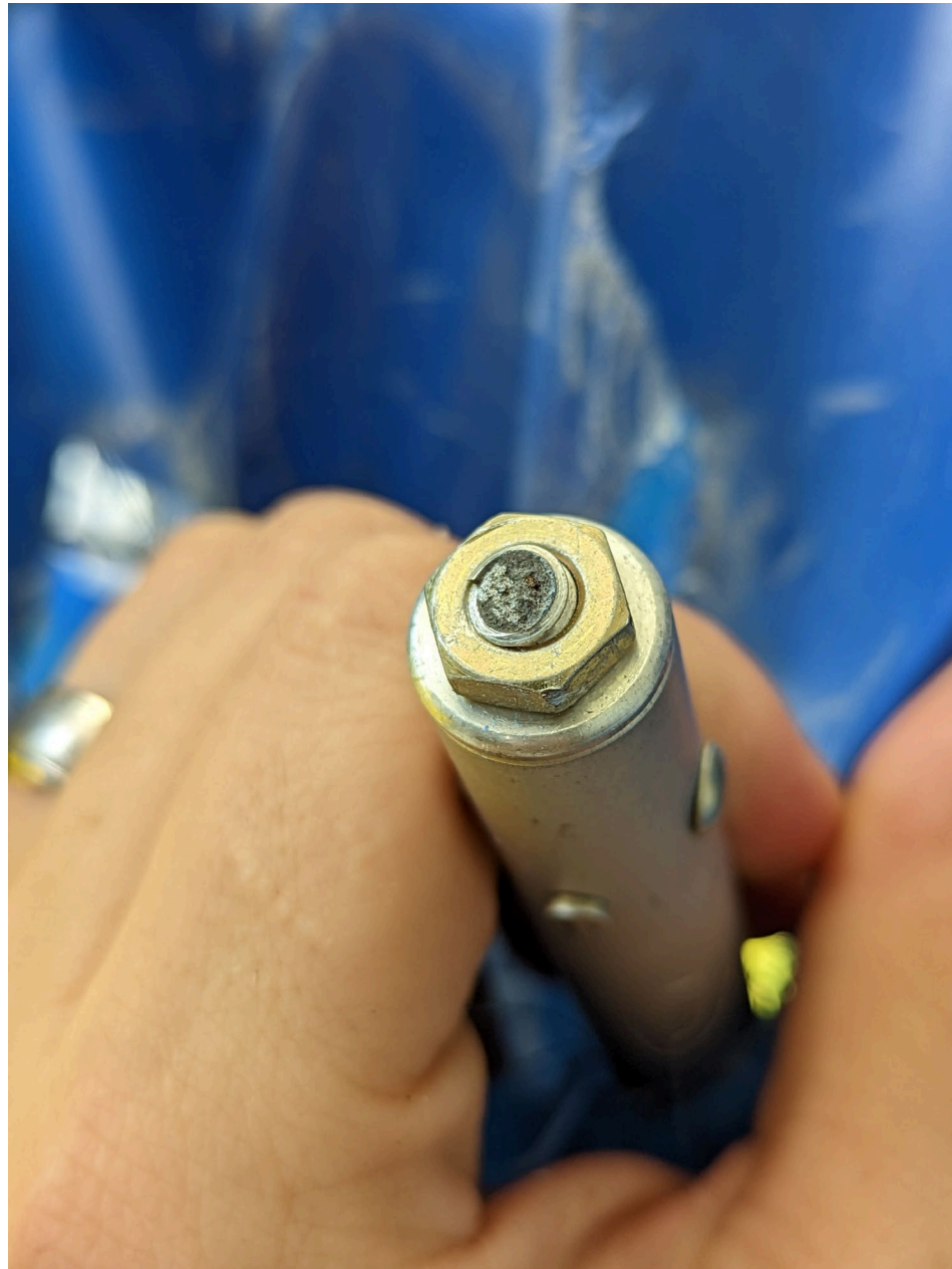
Photo 3 - Digital Photograph From Lockwood Aviation. View Showing the Impact Damaged Right Aileron Rod End.
