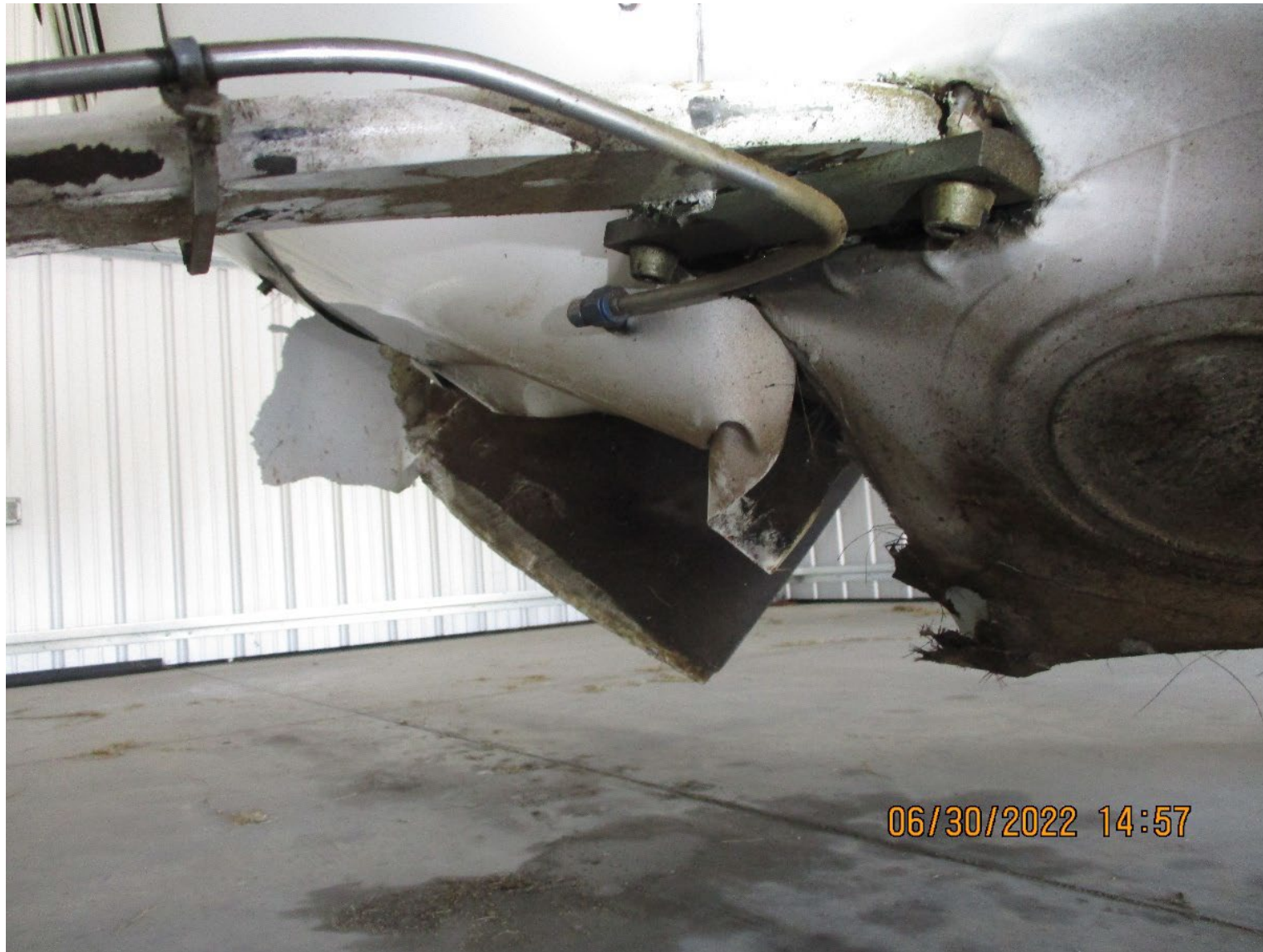
Photo 3: Accident airplane, left wheel strut damage, aft view. (Photo Courtesy of FAA)
