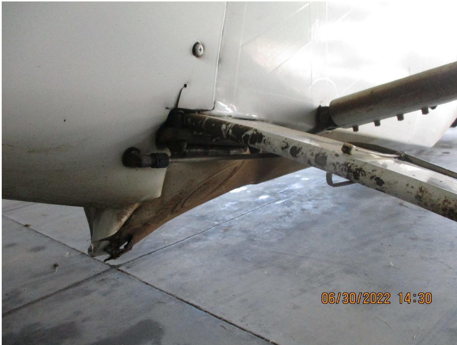
Photo 2: Accident airplane, left wheel strut damage, forward view. (Photo Courtesy of FAA)
