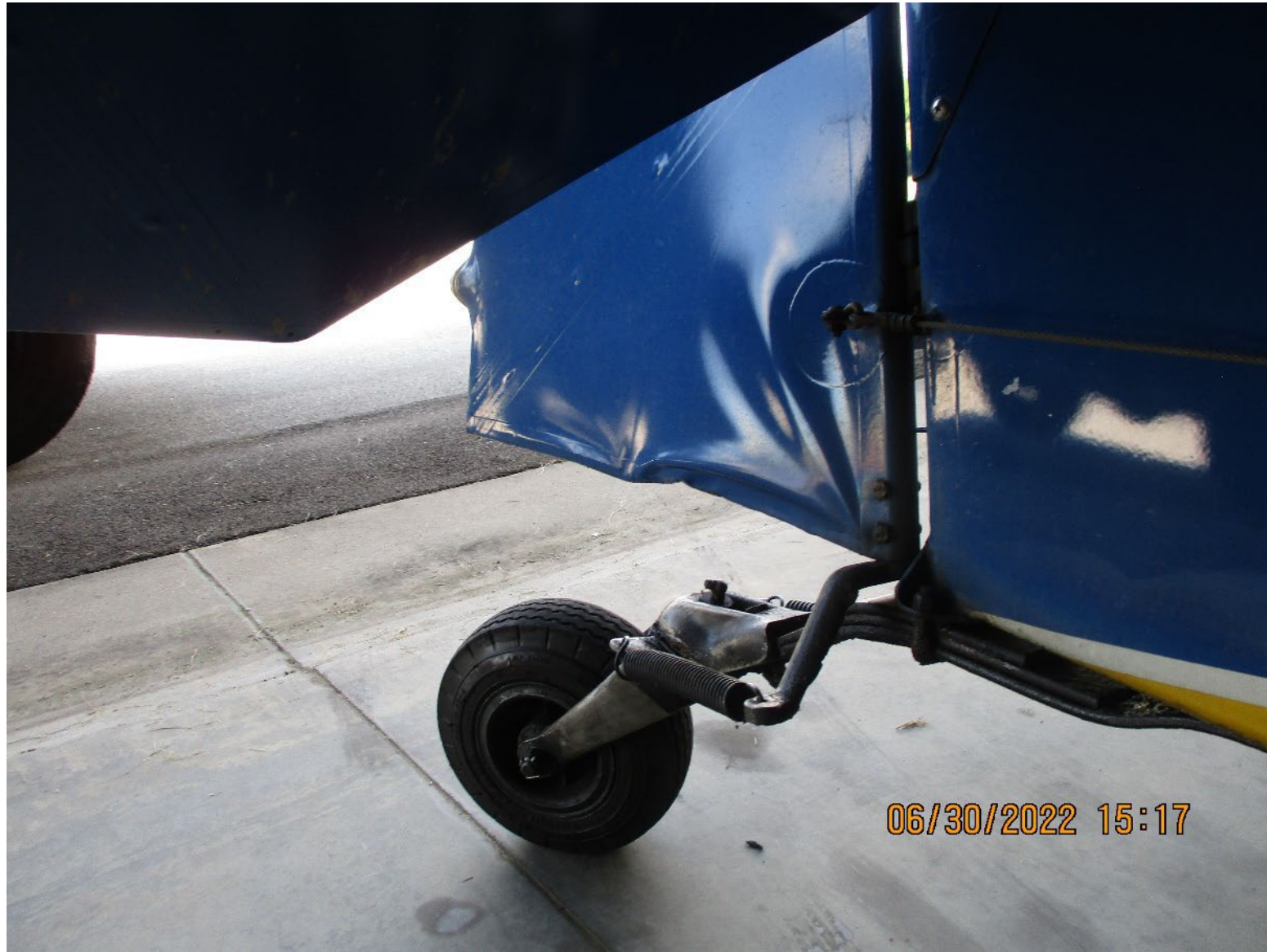
Photo 6: Accident airplane, rudder damage. (Photo Courtesy of FAA)
