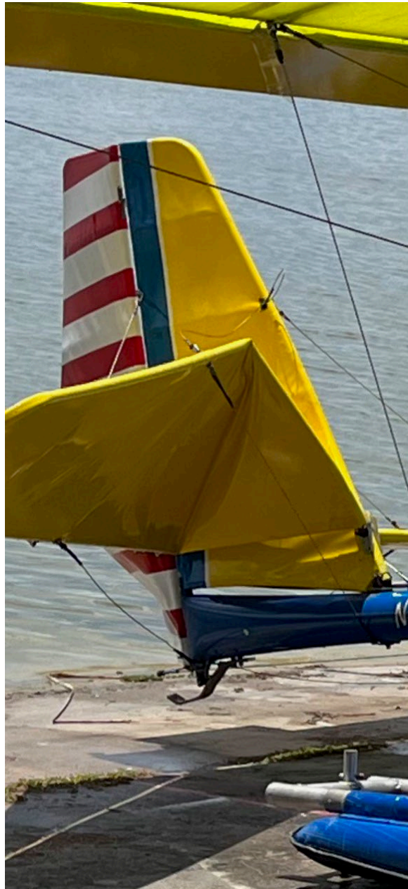
Photo 1 – FAA photo- Right horizontal damage
