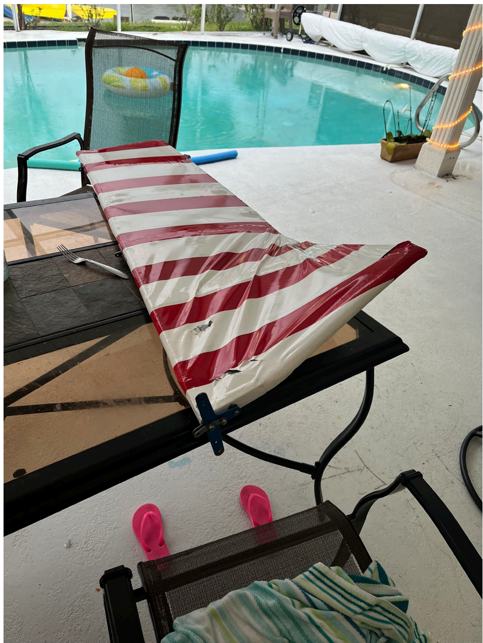
Photo 2 – FAA Photo-Rudder damage
