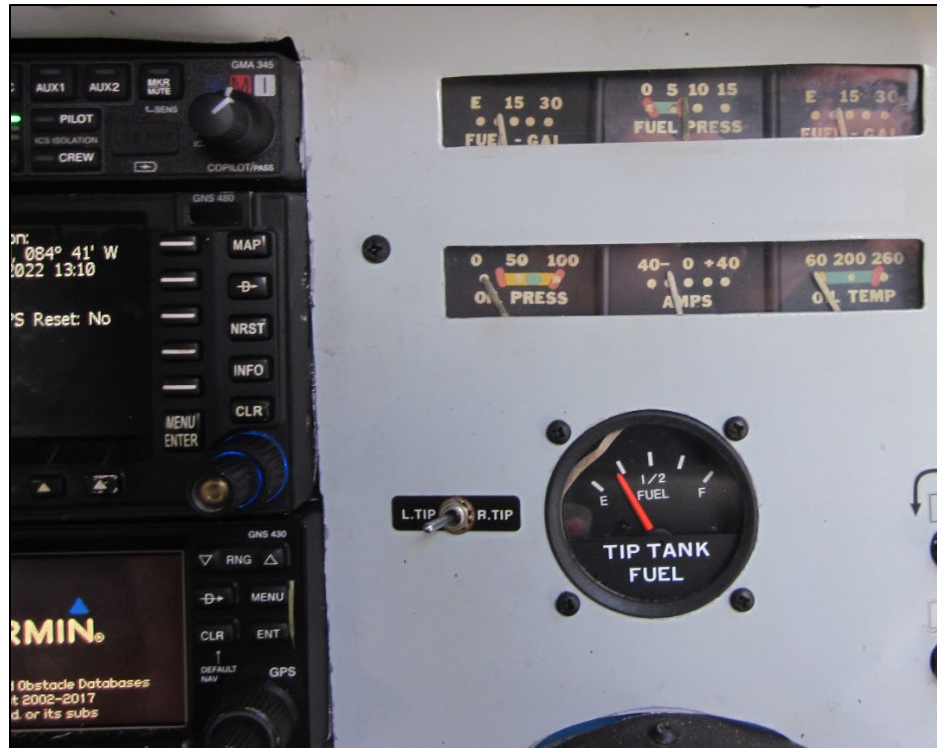
Figure 5: View of the fuel instrumentation, with power turned on to the aircraft (FAA Photograph)
