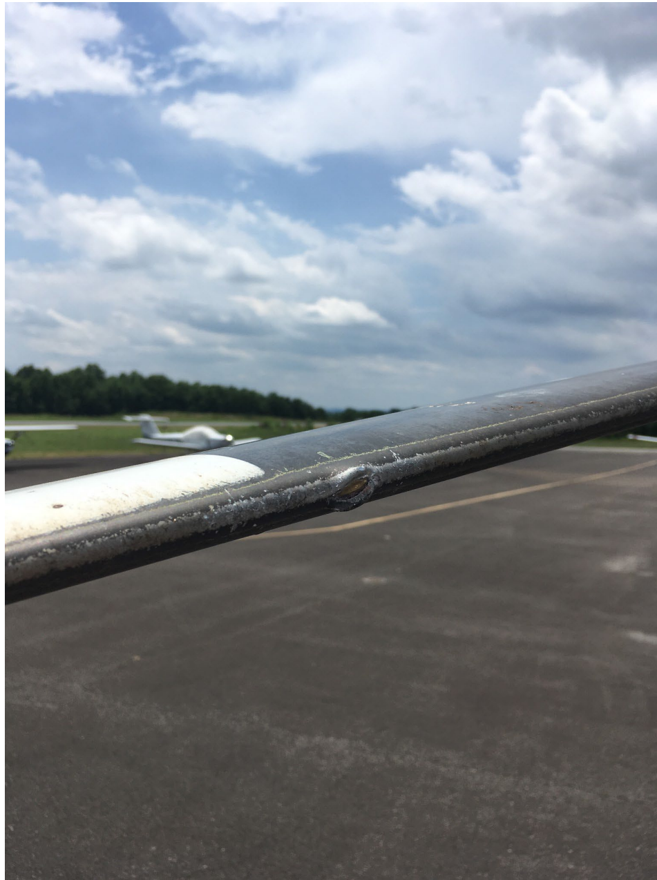
Photo 1 – View of main rotor blade damage (Courtesy of FAA)
