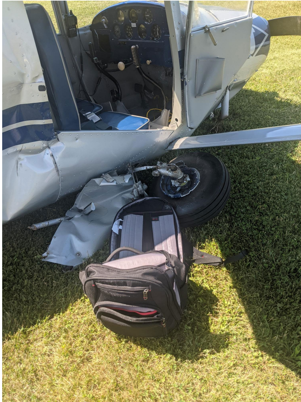
Photo 2 – main landing gear separated, (FAA)
