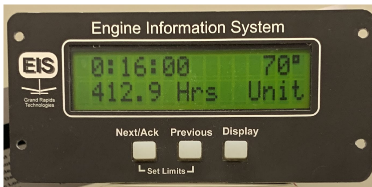
Figure 1. Flight Timer and Hourmeter parameters.
