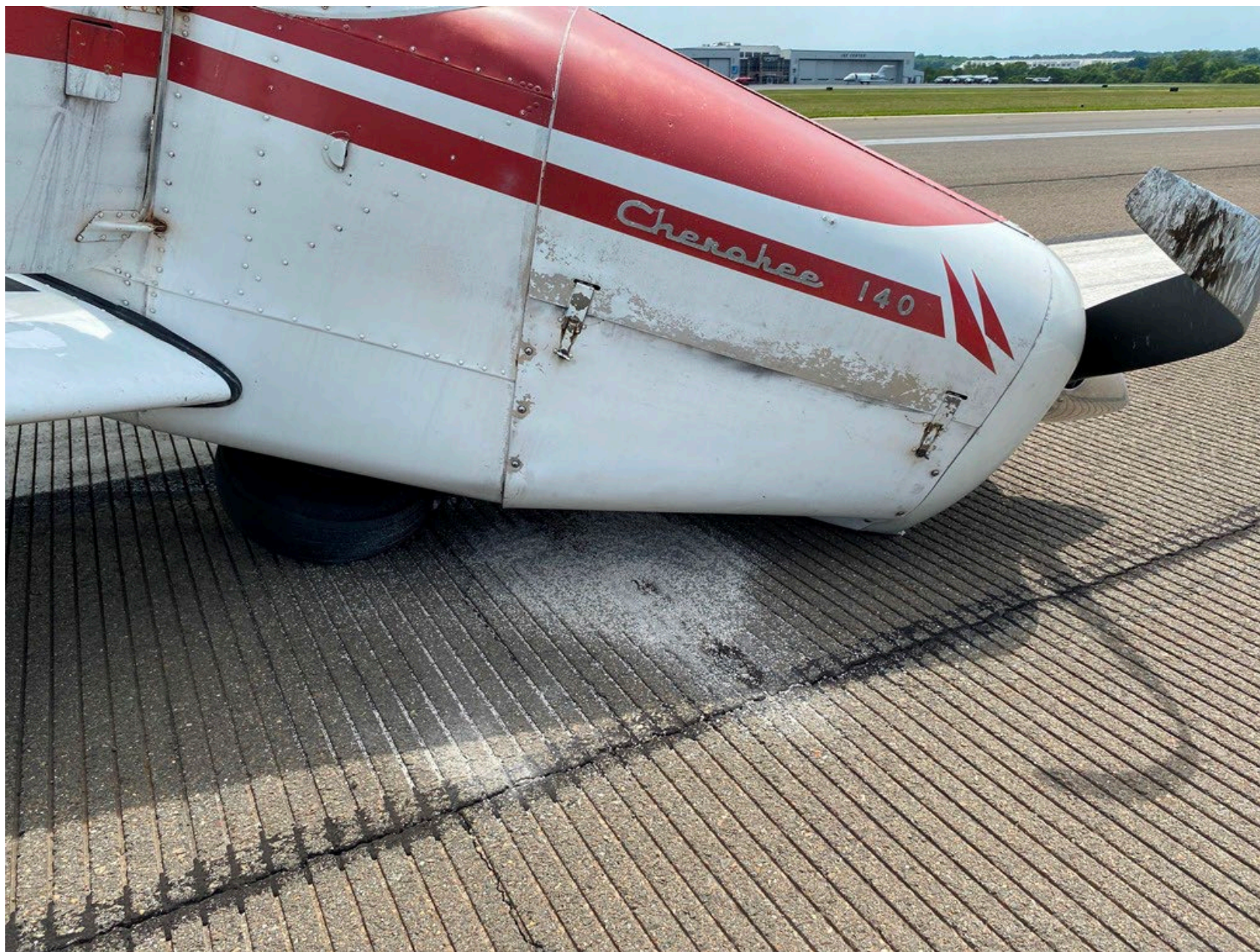
Photo 2 – External Damage to the Forward Engine Area on Right Side (FAA)
