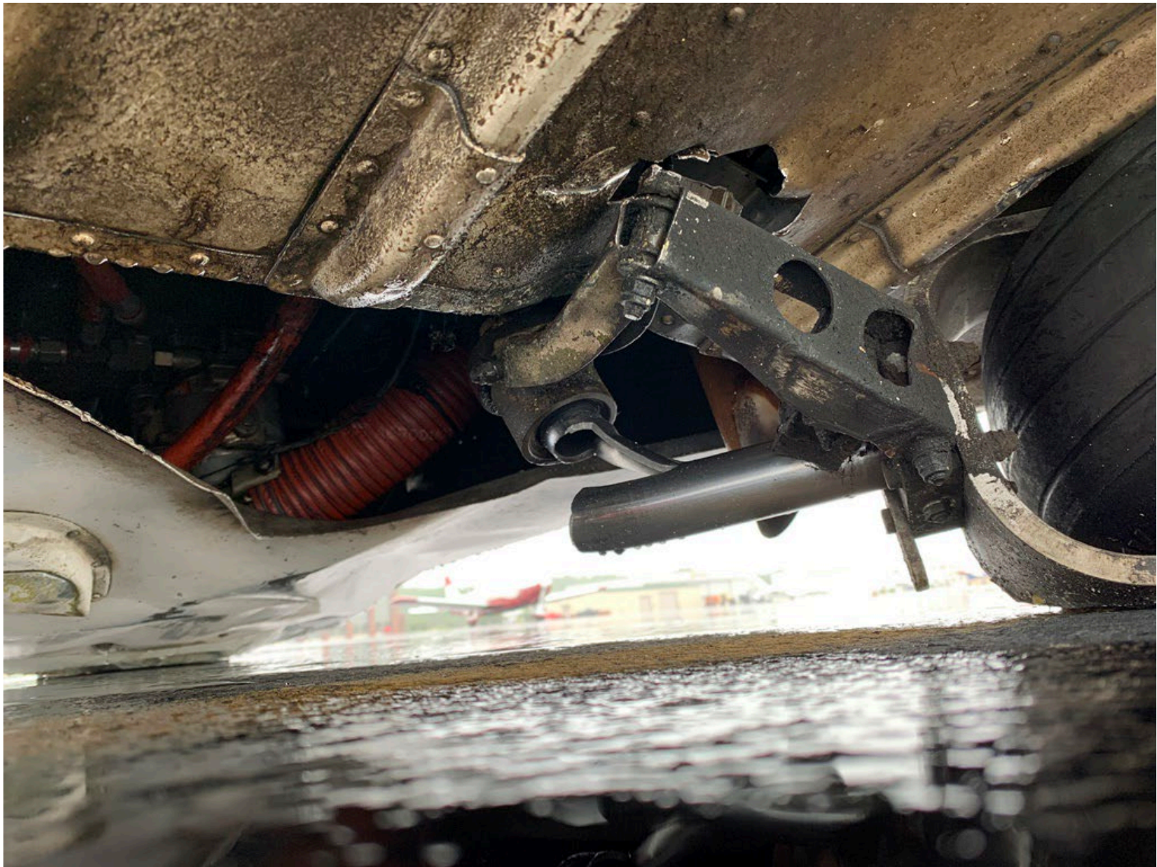
Photo 3 – Damage Aft of the Firewall (FAA)
