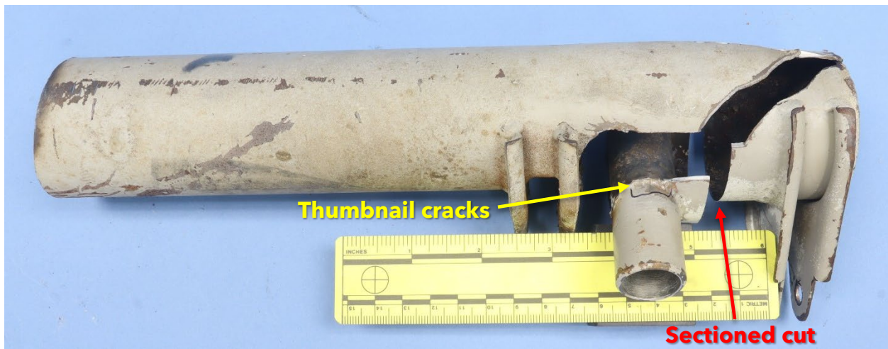
Figure 4. View of the torque tube after sectioning to reveal the crack faces. The location of the thumbnail cracks and sections are annotated in the figure.
