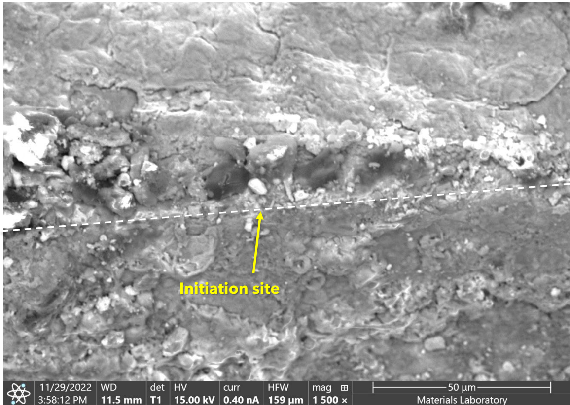
Figure 15. BE micrograph of a closer view of the edge of the crack in Figure 4, with the edge annotated and the fatigue crack initiation site labeled.
