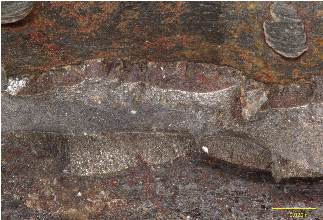
Figure 8. Closer view of some of the thumbnail cracks in the middle of the fracture in Figure 7.
