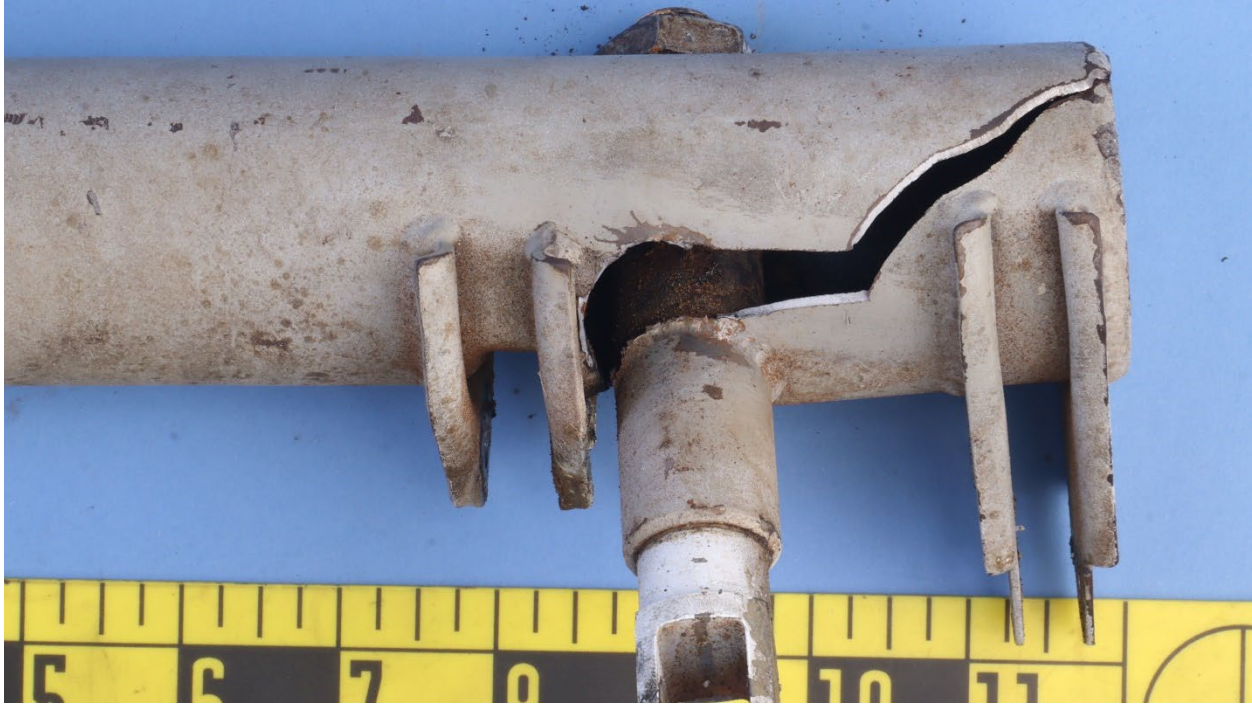
Figure 3. Closer view of the fracture near the weld along the boss of the torque tube.
