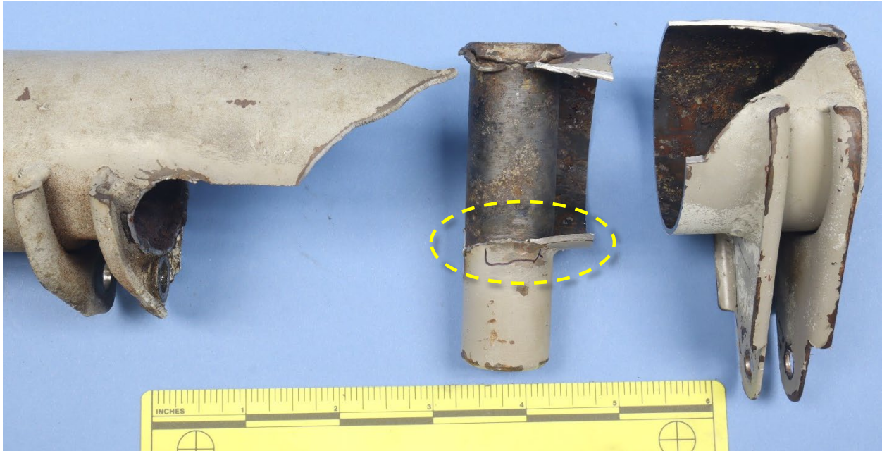
Figure 5. The sectioned portions of the torque tube, with the different sections separated to expose the tube interior.
