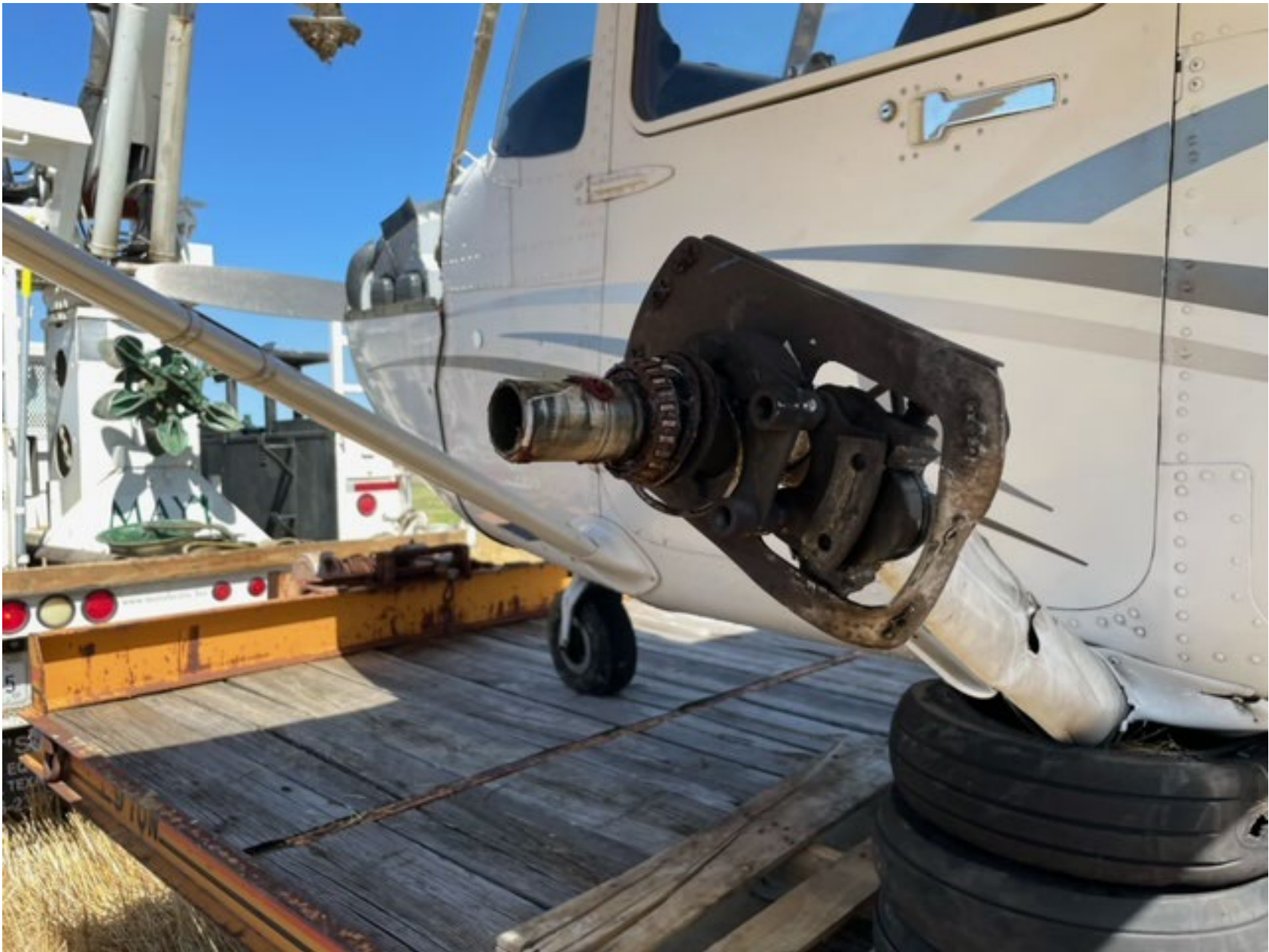
Photo 2 – View of the damaged left main landing gear.
