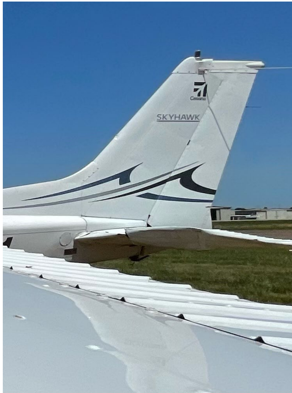
Photo 1 – View of right horizontal stabilizer damaged
