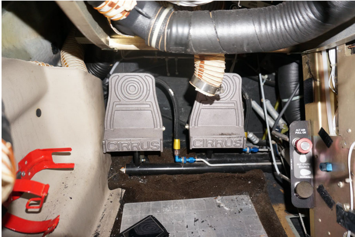
Photograph 7 - Pilot Side Rudder Pedals and Brake Lines
