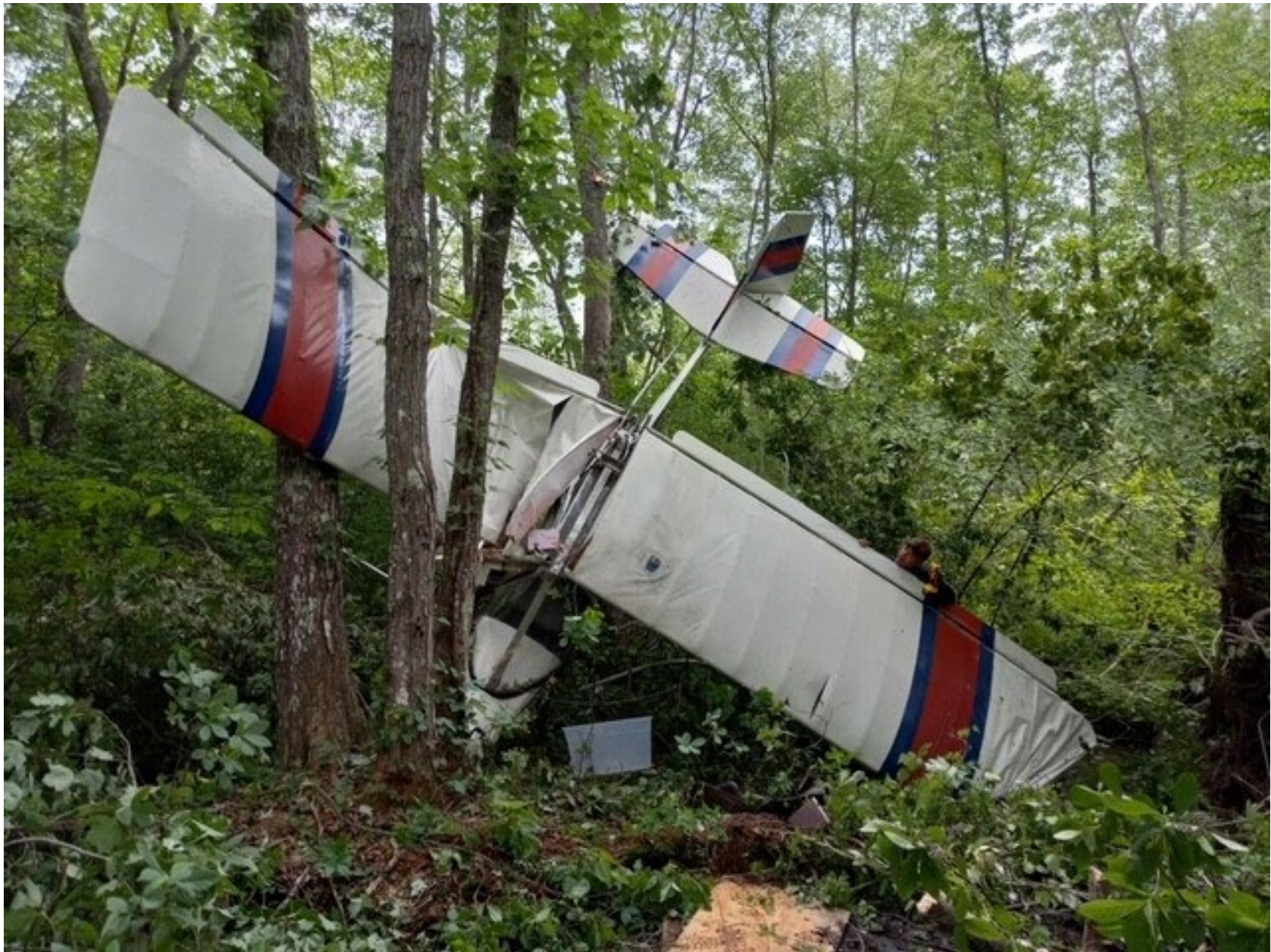
Photo 1 – Digital Photograph From Owner. Front View of Top of Airplane at the Accident Site. Note the Substantial Damage to the Right Wing.
