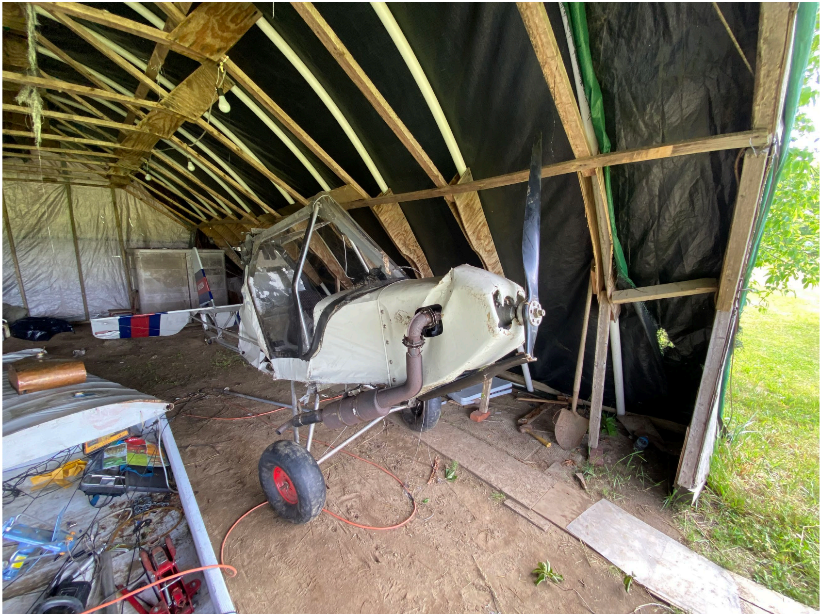
Photo 3 – FAA Digital Photograph. Right Forward Quartering View of the Airplane Following Recovery. Note the Damage to 1 Propeller Blade and Slight Damage to the Other Propeller Blade.
