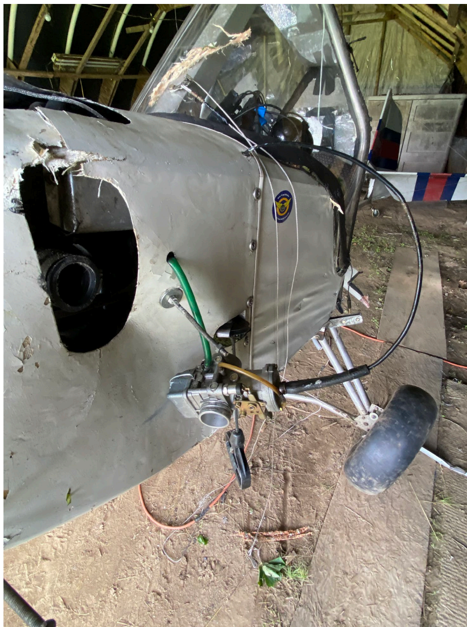
Photo 4 - FAA Digital Photograph. Left Forward Quartering View of the Airplane Following Recovery. Note the Separated Single Carburetor.
