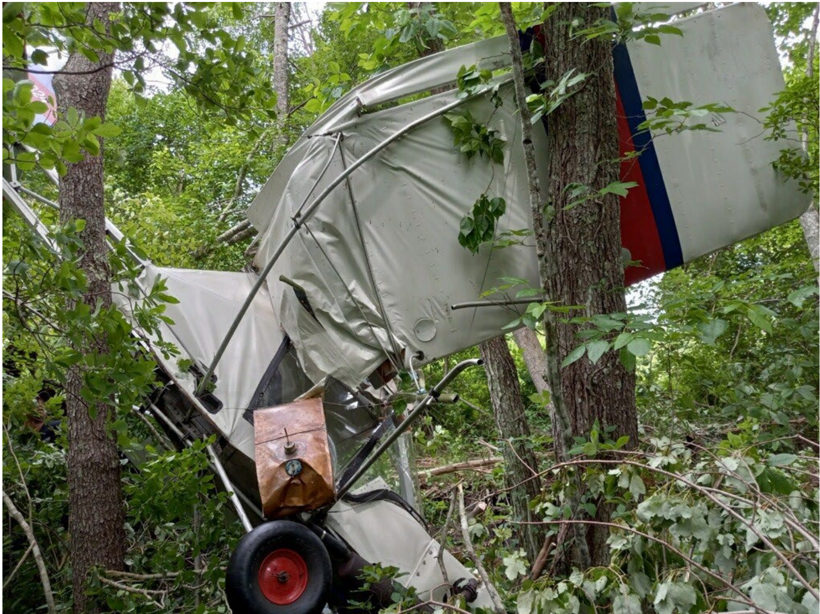
Photo 2 - Digital Photograph From Owner. Right Side View of The Airplane at the Accident Site. Note the Substantial Damage to the Right Wing.
