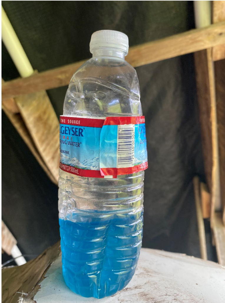
Figure 2: FAA Digital Photograph. View of Fuel Sample From Wing Fuel Tank Taken During Postaccident Examination.
