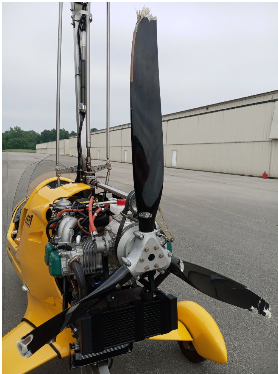
Photo 2 – Rear View of Gyro and Damage to Propeller (credit M. Beighey)
