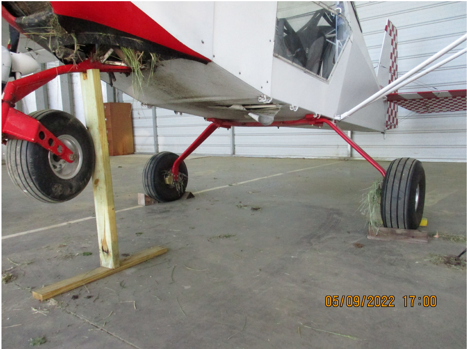
Photo 3 – View of nose landing gear and fuselage damage. (Courtesy of FAA)
