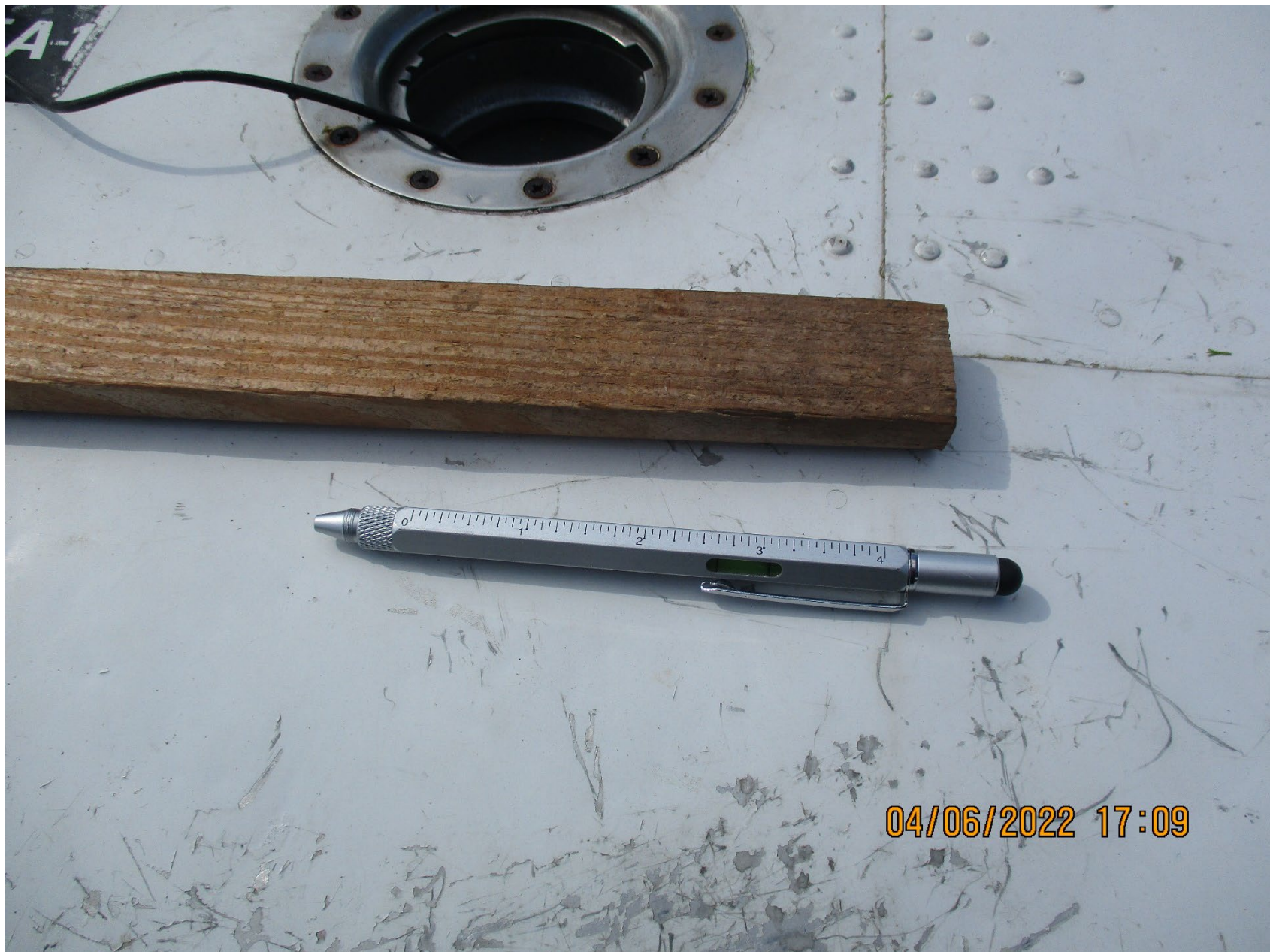
Photo 6 – View of Dry Fuel Measuring Stick Showing No Fuel (Photo Courtesy of FAA)
