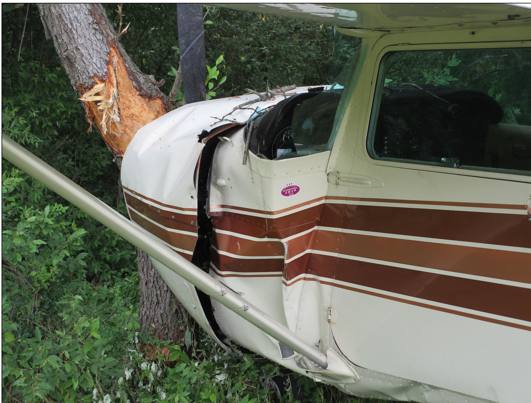
Photo 3: Overview of the nose, cowling section, and tree damage at the accident site (Photo Courtesy of FAA)
