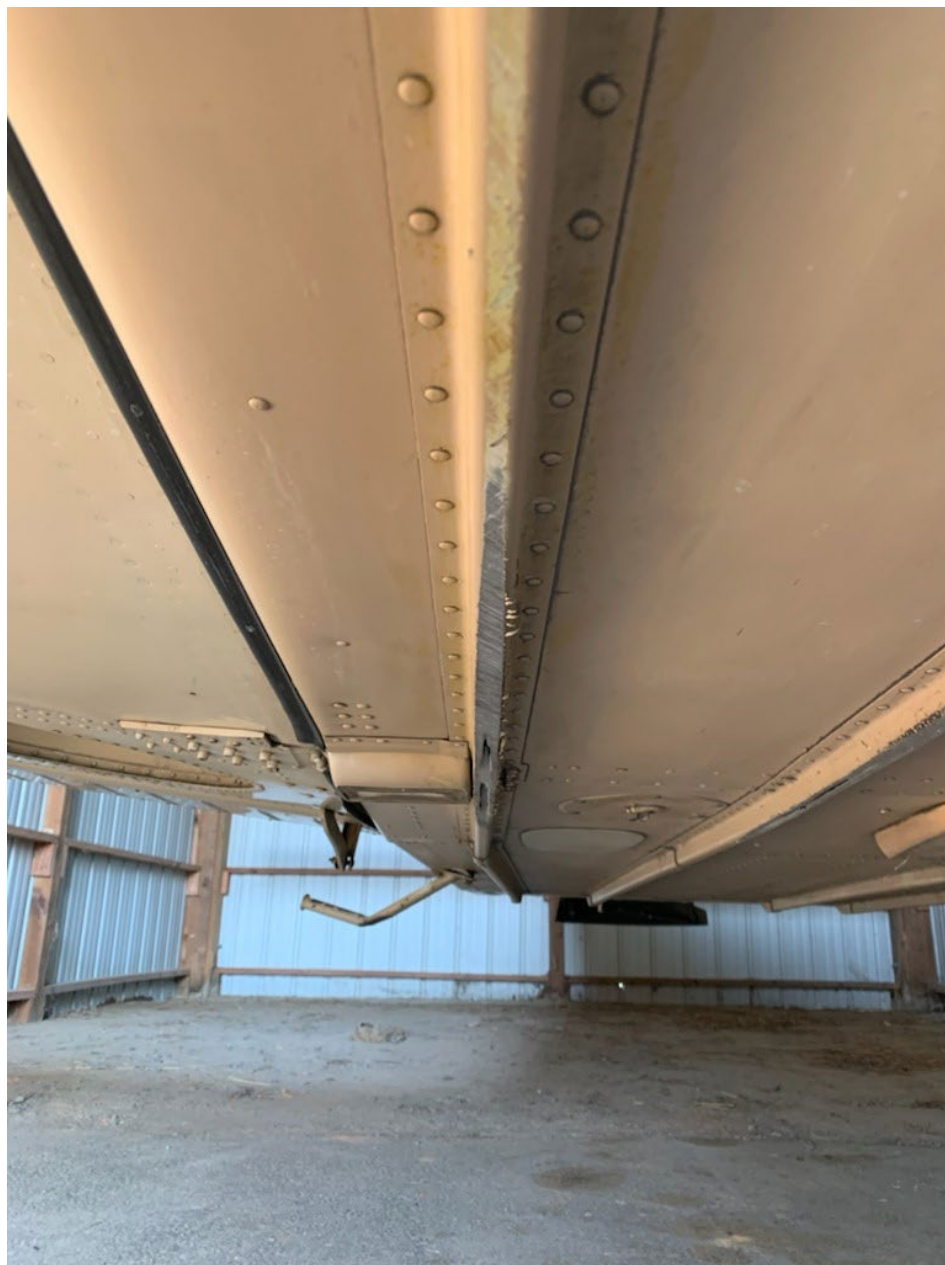
Photo 1 – external longerons (owner)
