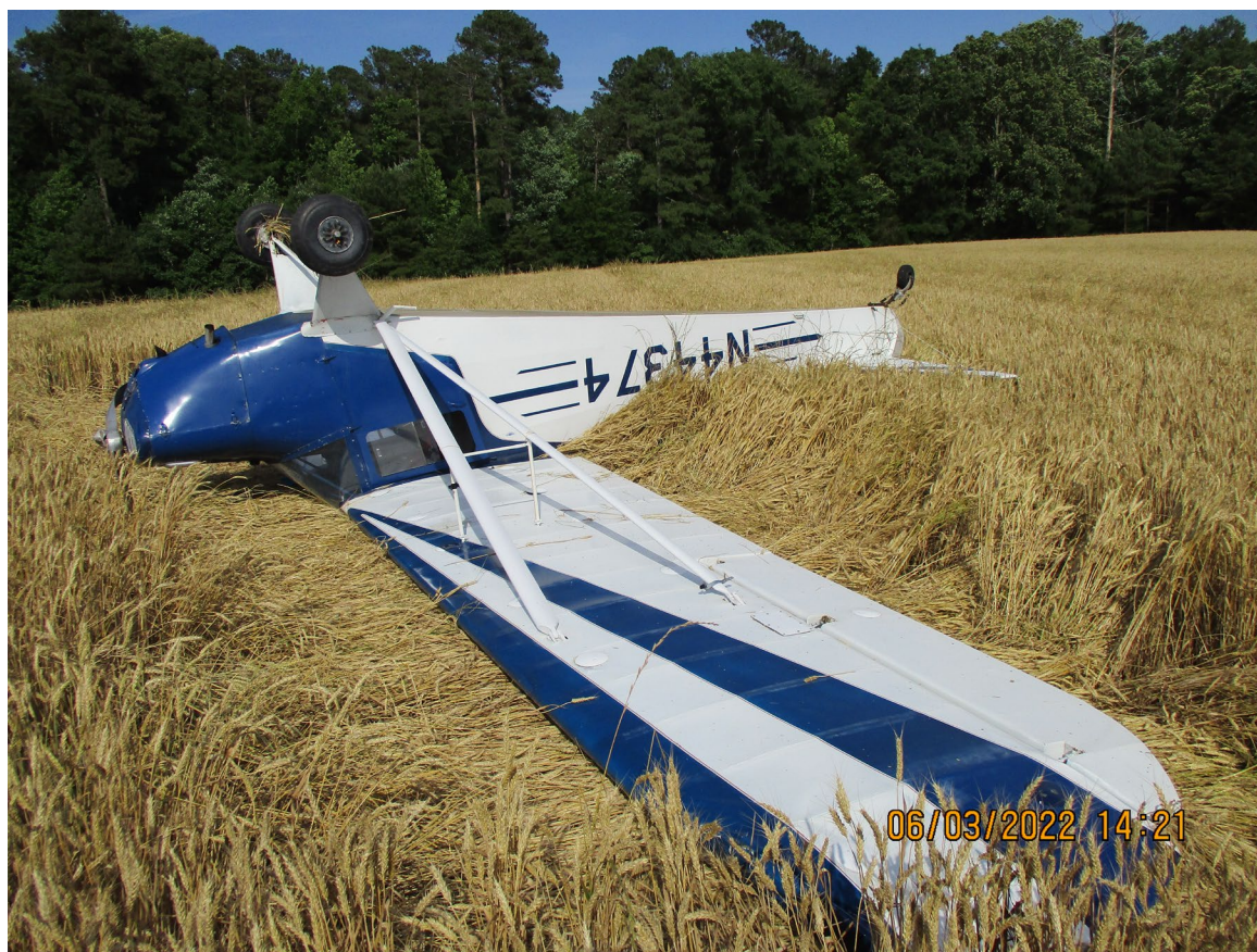
Photograph 1 - View of the airplane inverted where it came to rest. (Courtesy of FAA)
