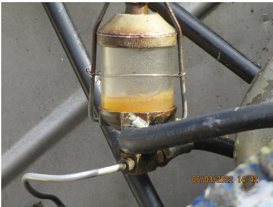
Photograph 2 - View of the gascolator. (Courtesy of FAA)
