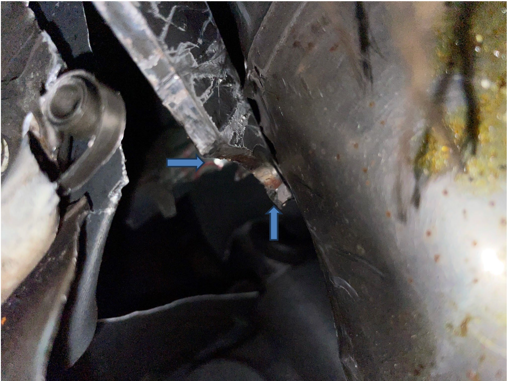
Photo 3 – View of Fractured Yoke Lug (Operator)
