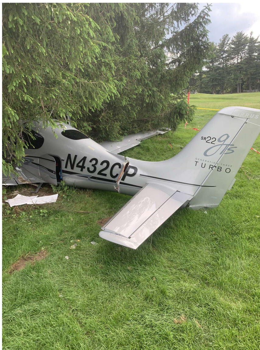
Photograph 1 - Left side of empennage showing hull damage (Courtesy of FAA)
