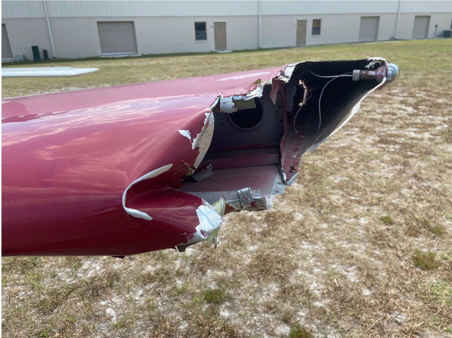
Photo 3 – Closeup view of damaged left wing. (Courtesy of FAA)
