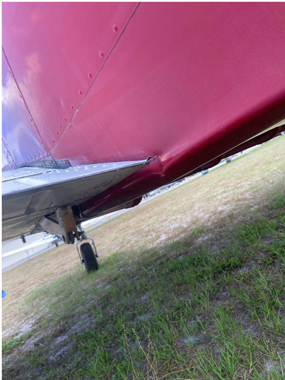
Photo 5 – View of left wing flap and fuselage crease. (Courtesy of FAA)
