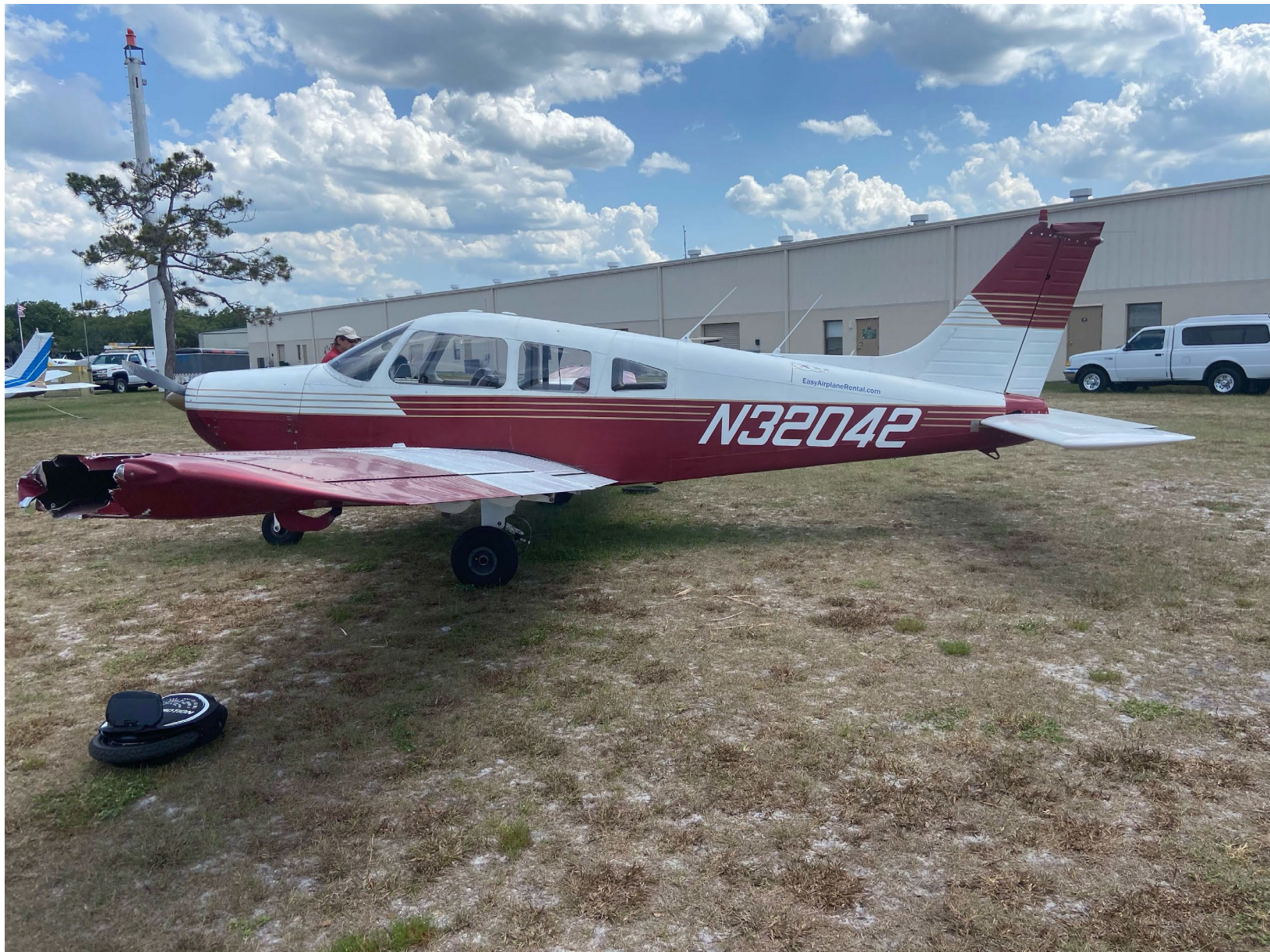
Photo 1 – Left profile view of airplane showing damaged left wing. (Courtesy of FAA)
