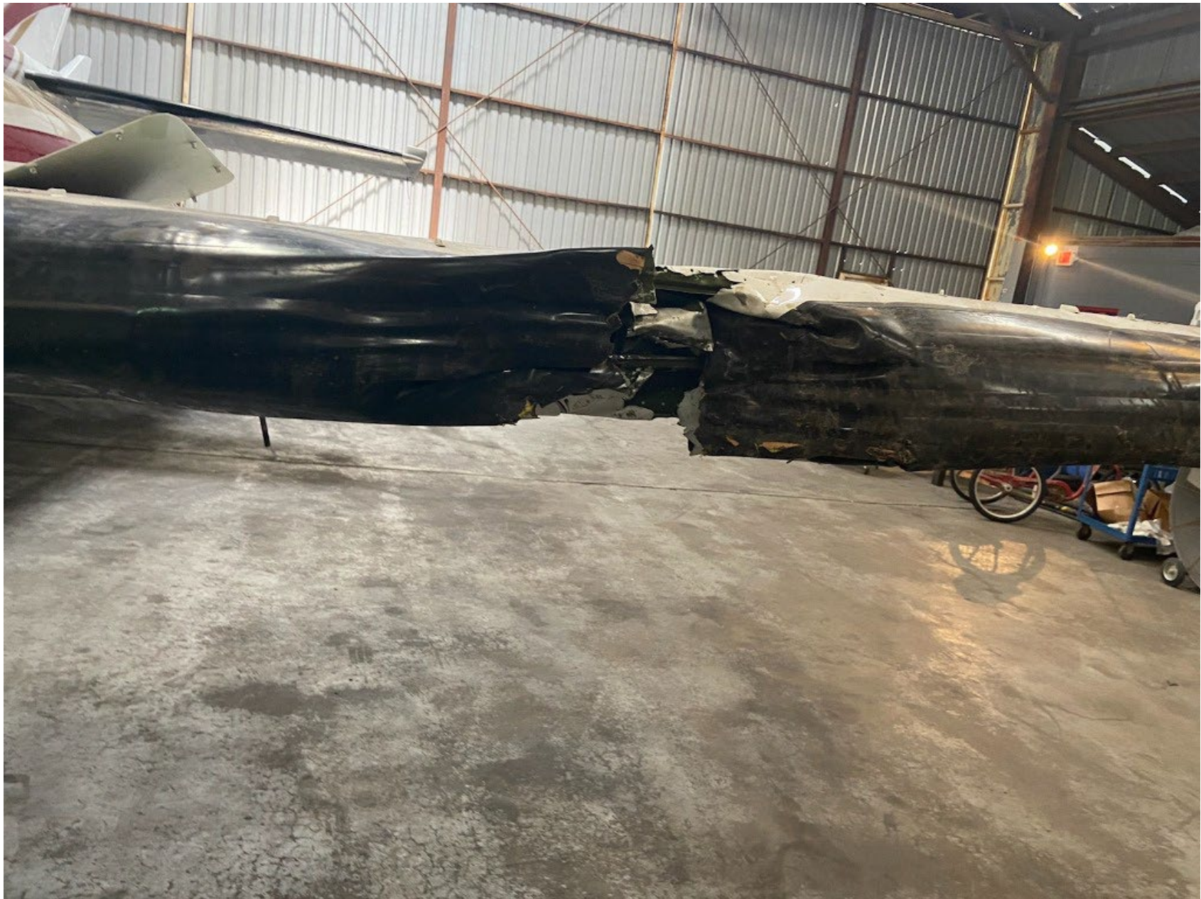
Photo 2 – Damage to the Leading Edge of the Left Wing (credit FAA)
