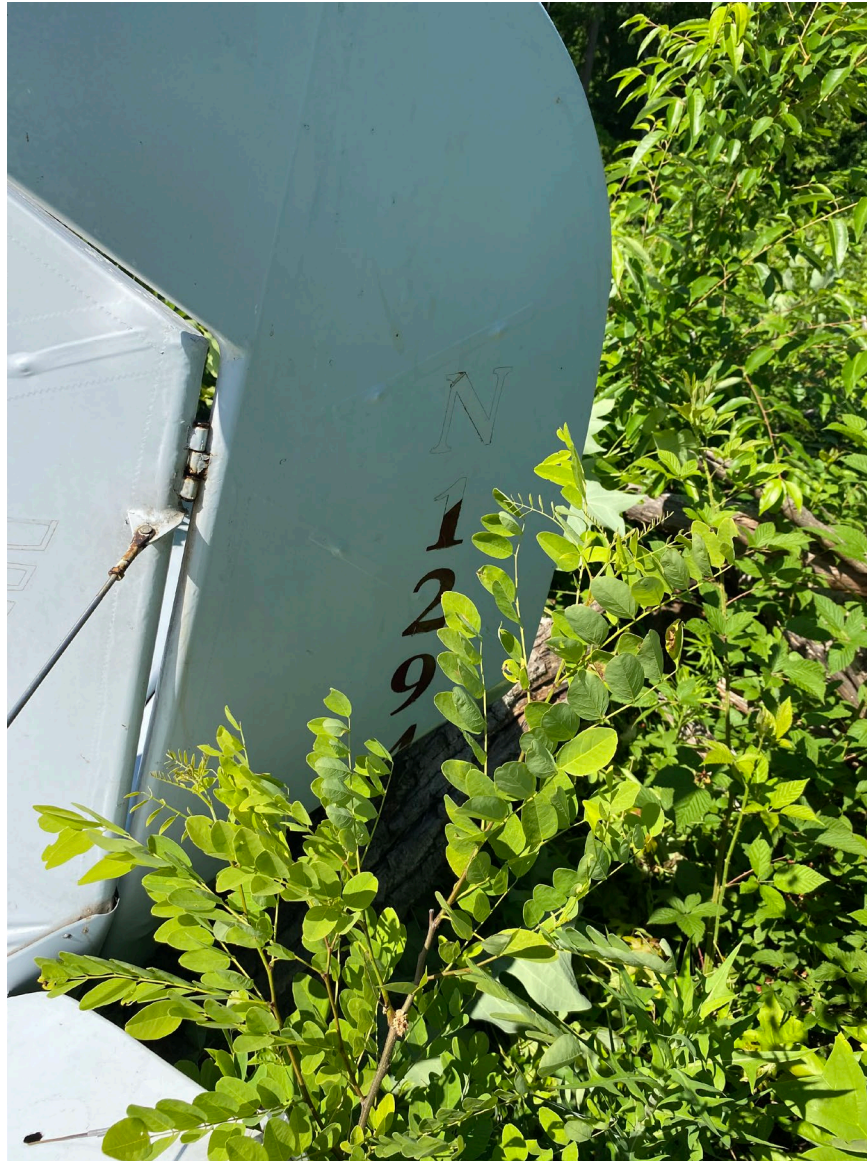
Photograph 3 - Rudder damage (Courtesy of FAA)
