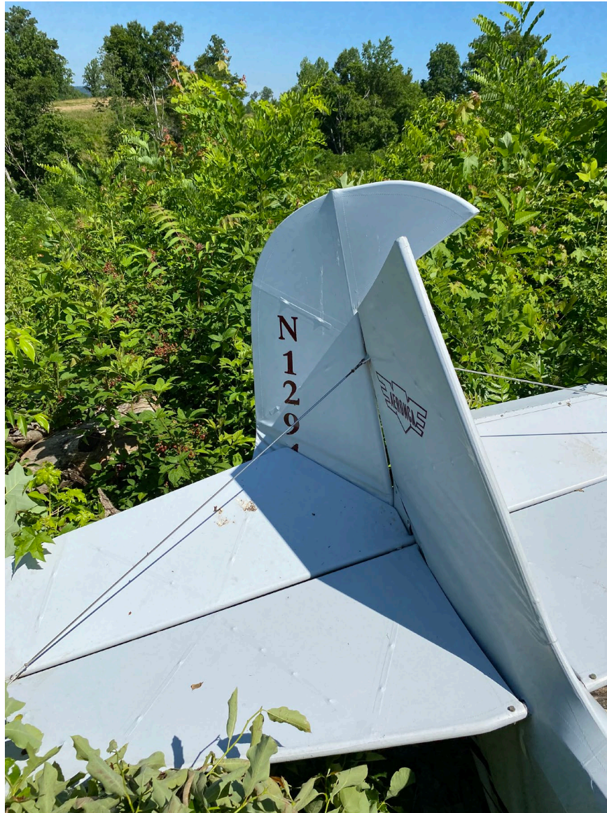
Photograph 2 - Rudder damage (Courtesy of FAA)
