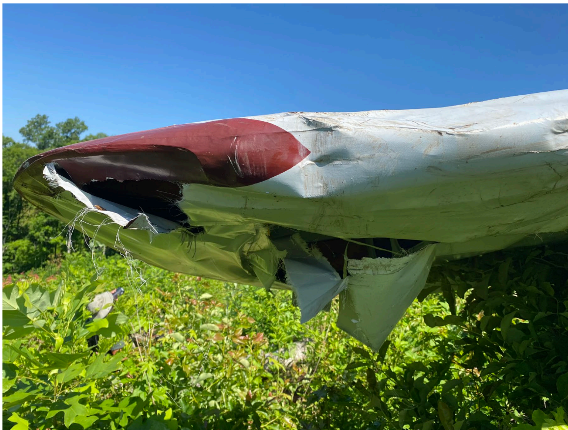
Photograph 5 - Right wing damage (Courtesy of FAA)
