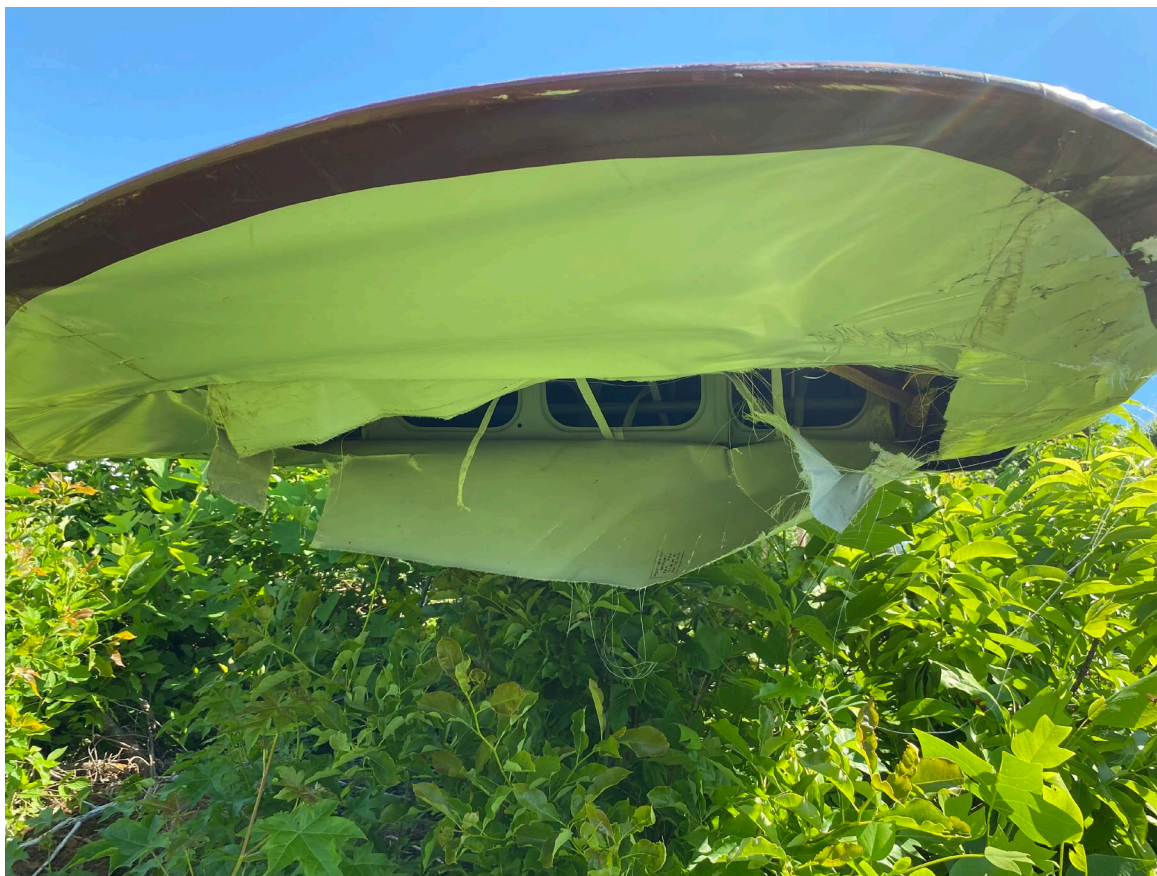
Photograph 4 - Right wing damage (Courtesy of FAA)
