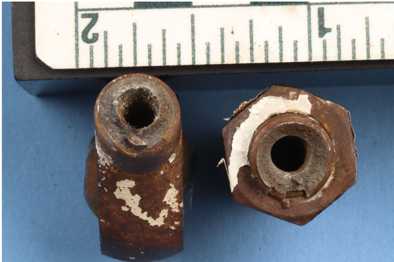
Figure 3. Slant fractures on fracture faces of connecting rod end fitting.
