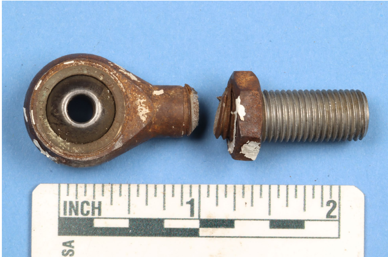
Figure 2. Two portions of connecting rod end fitting exhibiting plastic deformation above the stop nut.
