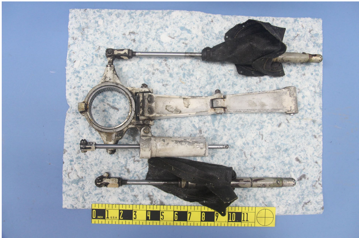
Figure 1. Left and right steering connecting rod assembly as received.
