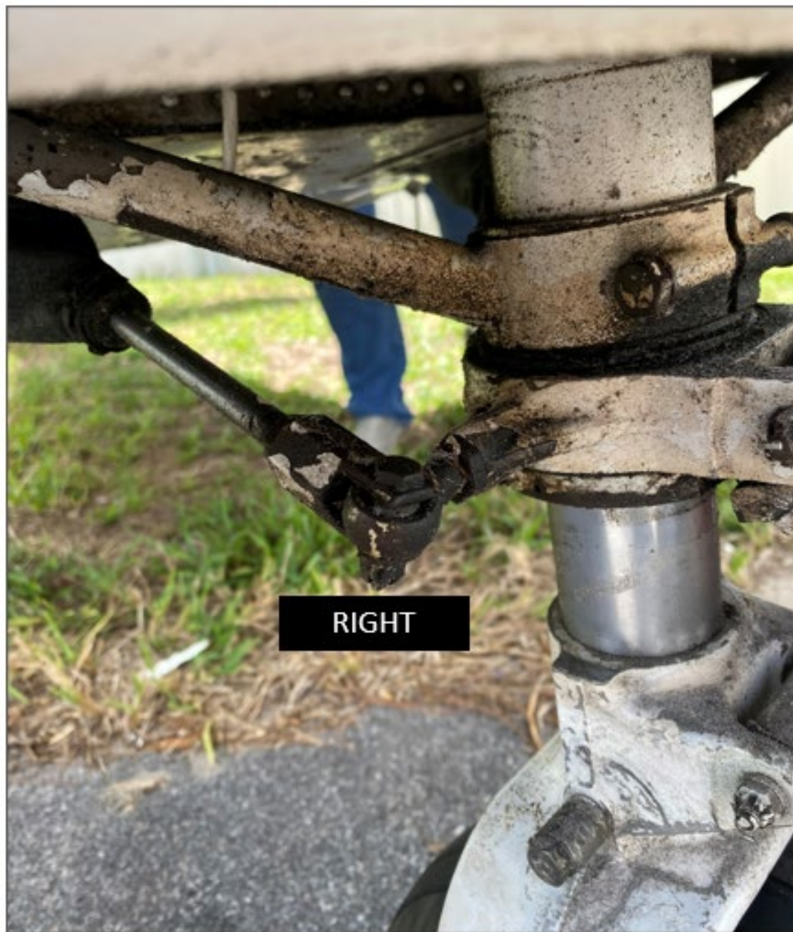
Photo 5: Overview of the right steering connecting rod remaining connected (Photo Courtesy of FAA)
