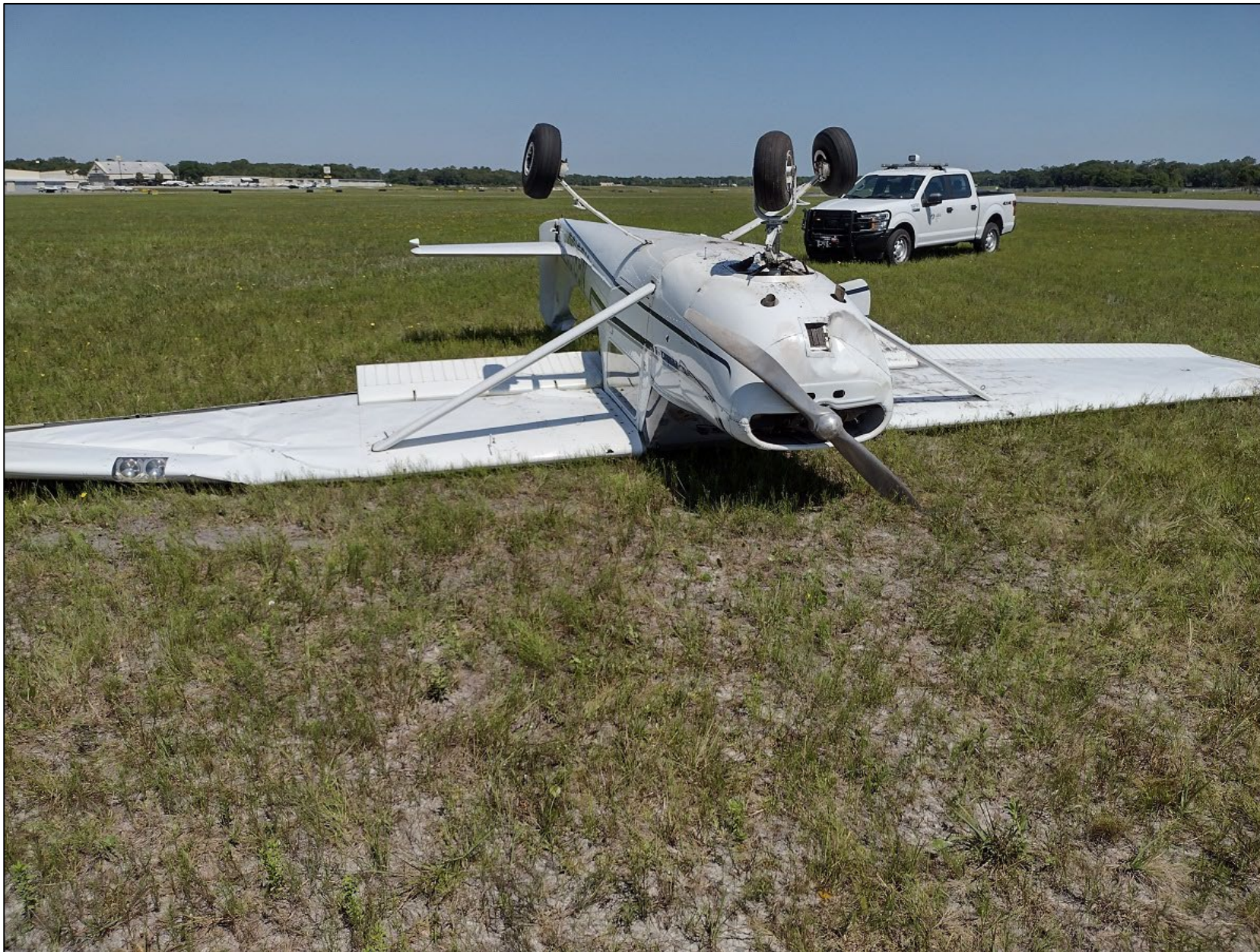
Photo 1: Overview of the substantial damage sustained to the airplane's right wing (Photo Courtesy of FAA)
