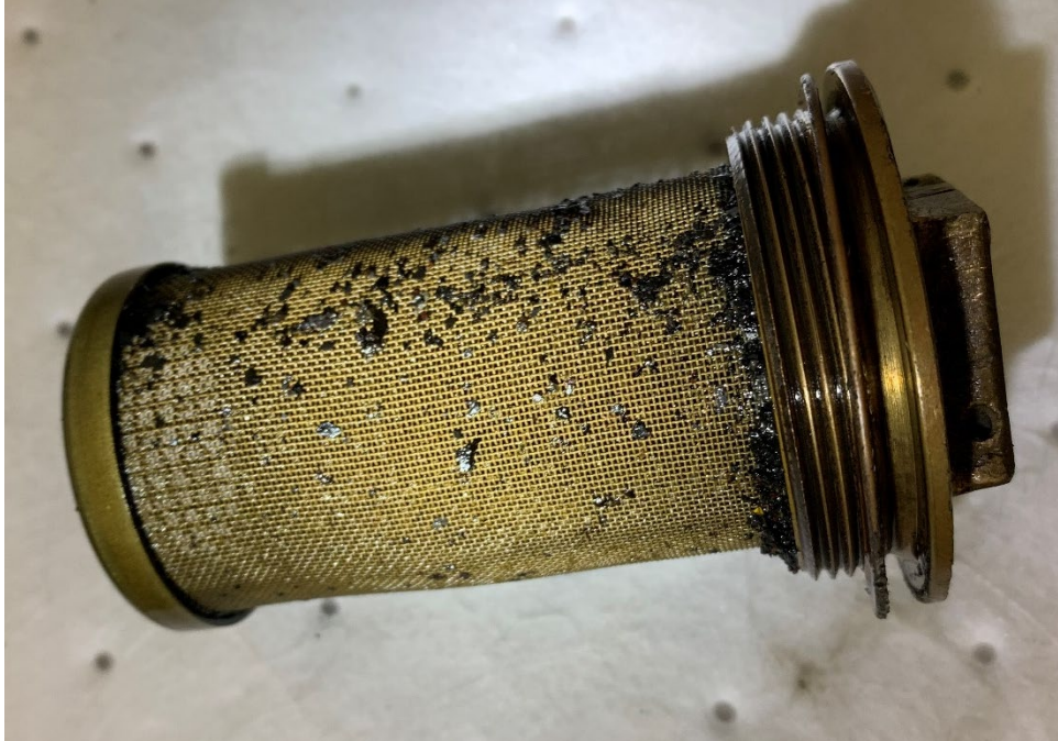
Figure 16. View of oil suction screen.
