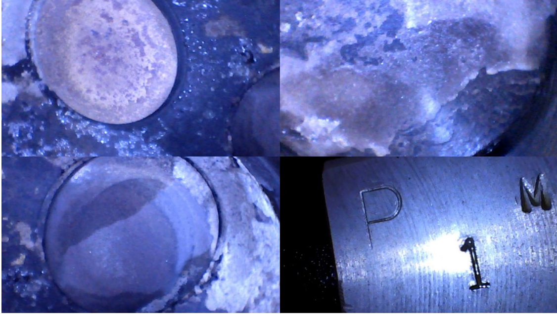
Figure 9. View of No. 1 cylinder piston face and valve faces.
