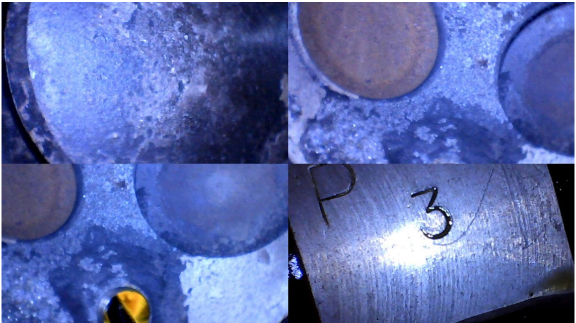
Figure 10. View of No. 3 cylinder piston face and valve faces.
