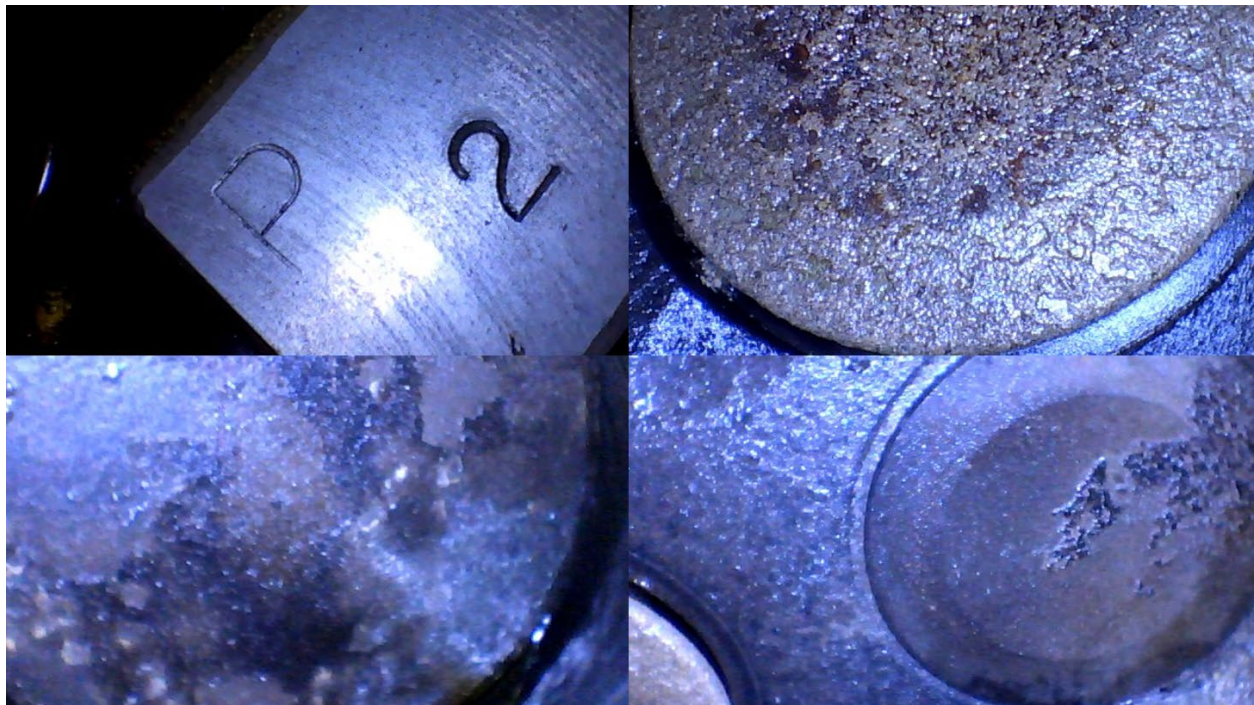
Figure 12. View of No. 2 Cylinder piston face and valve faces.
