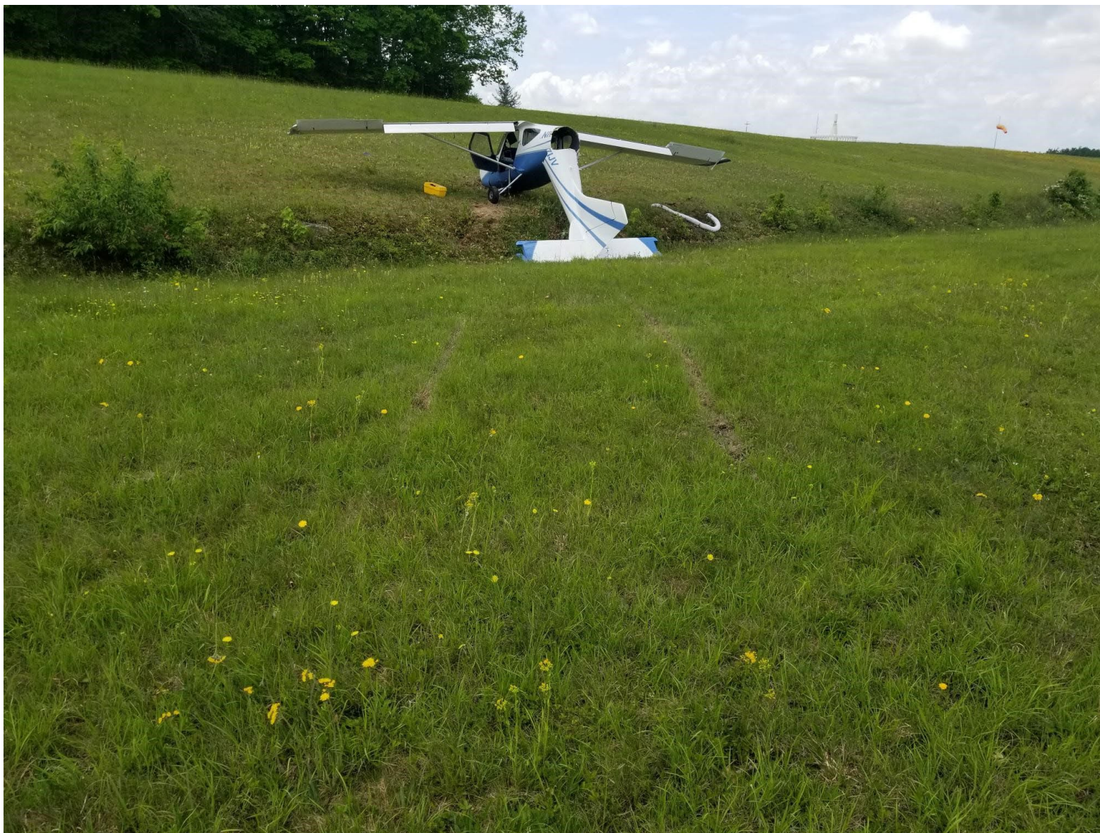
Photo 1 – View of airplane wreckage showing damage to fuselage. (Courtesy of FAA)
