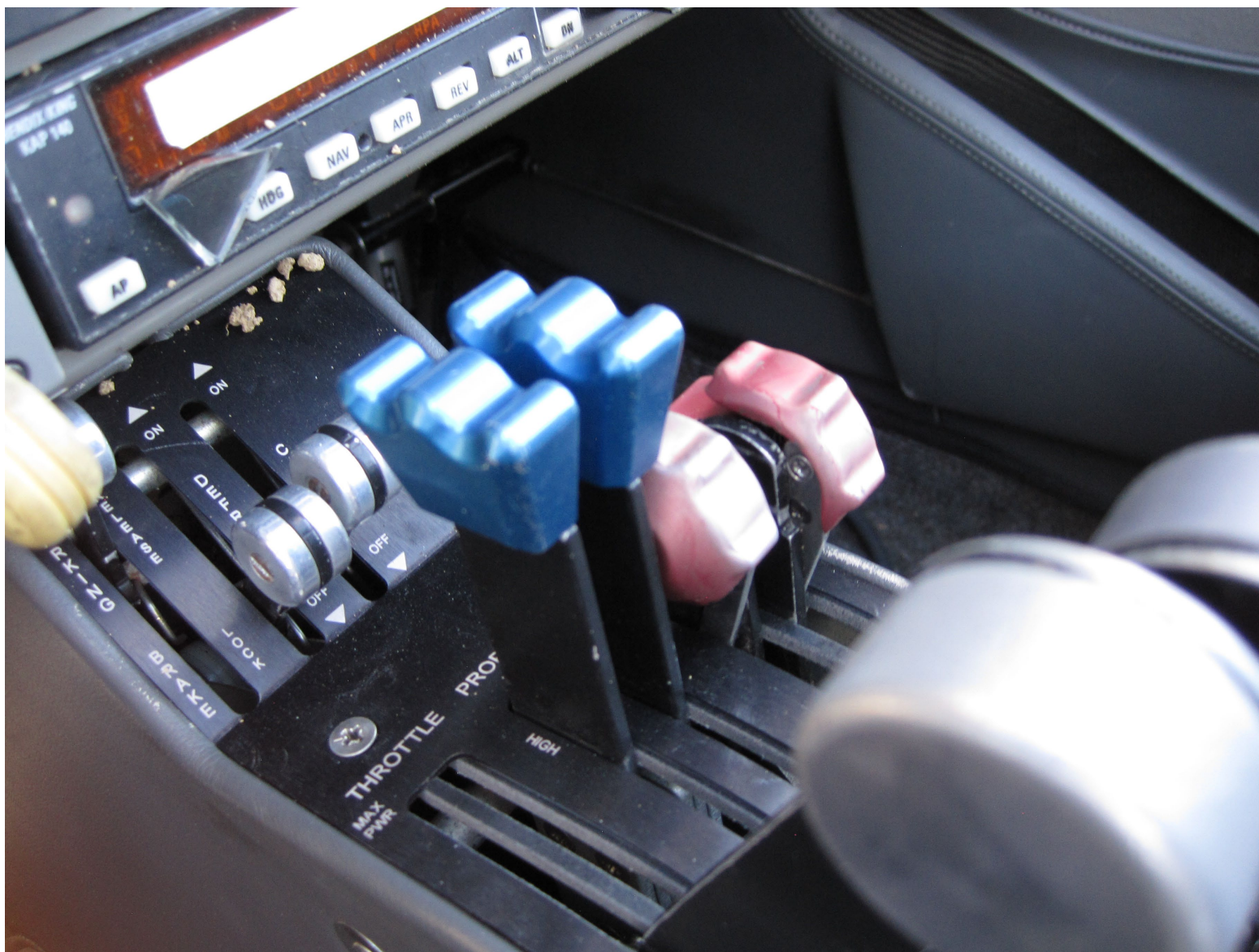
Photograph 3 - Propeller and Mixture Controls (Courtesy of FAA)
