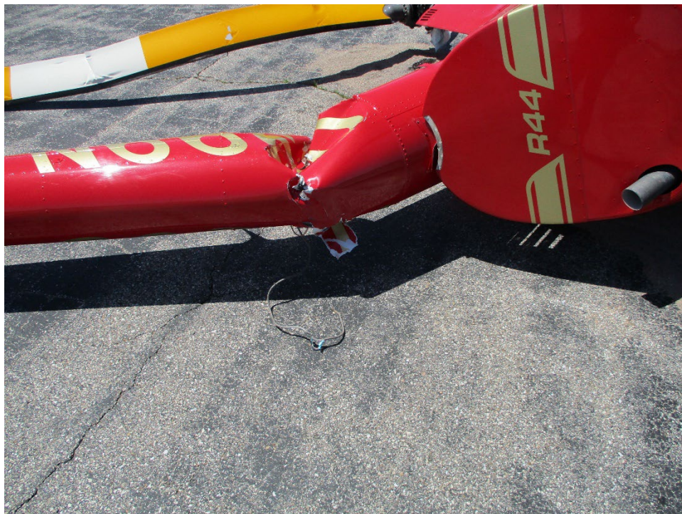
Photograph 3 – Accident helicopter – Damaged tail boom of helicopter.
