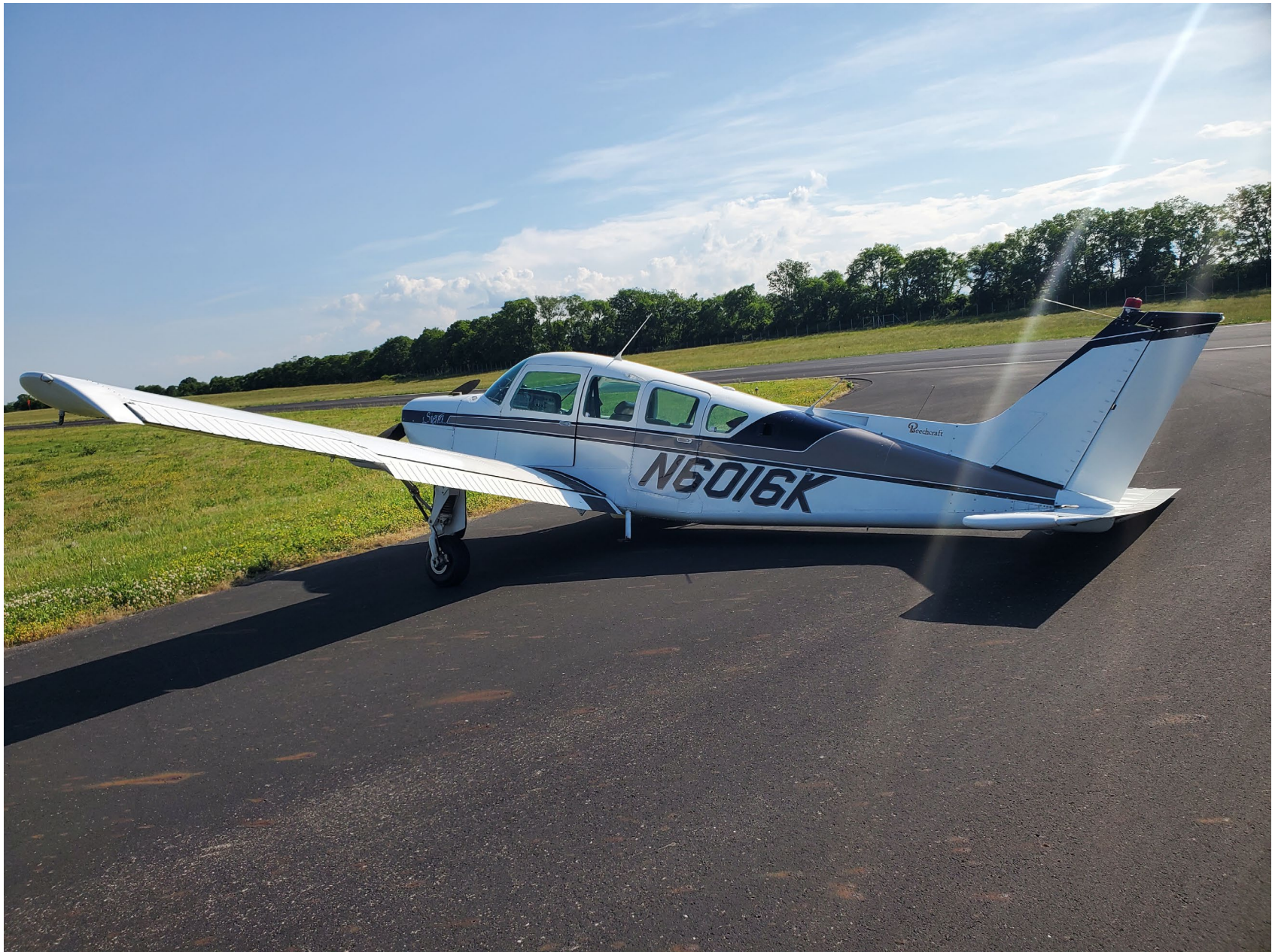
Photo 1 – Digital Photograph From Pilot. Left Side View of the Airplane Where it Came to Rest. Note the Collapsed Right Main Landing Gear.
