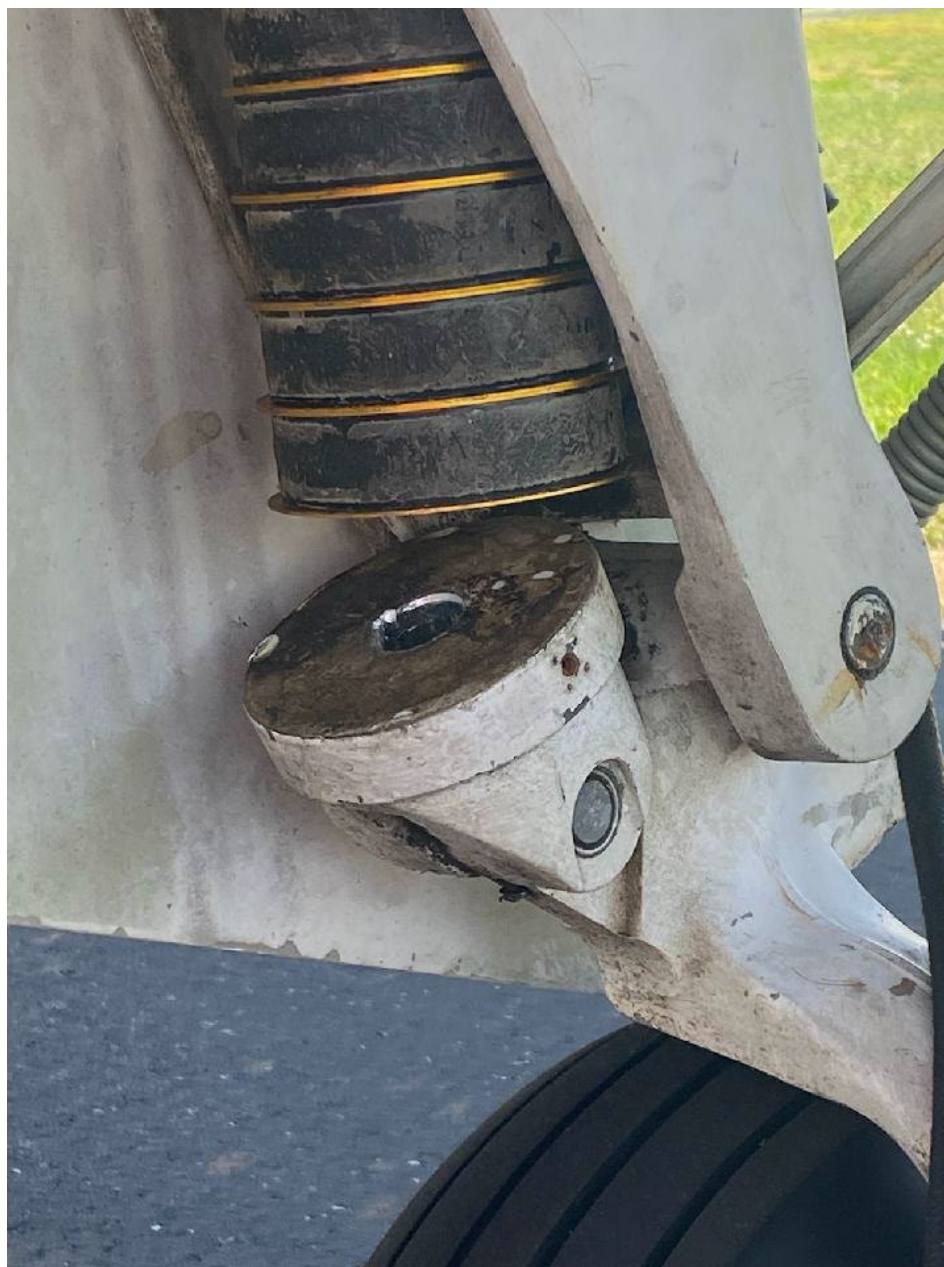
Photo 5 - Digital Photograph From Pilot. View Showing the Separation of the Right Main Landing Gear Shock Absorber Rod From the Compressor Fitting.
