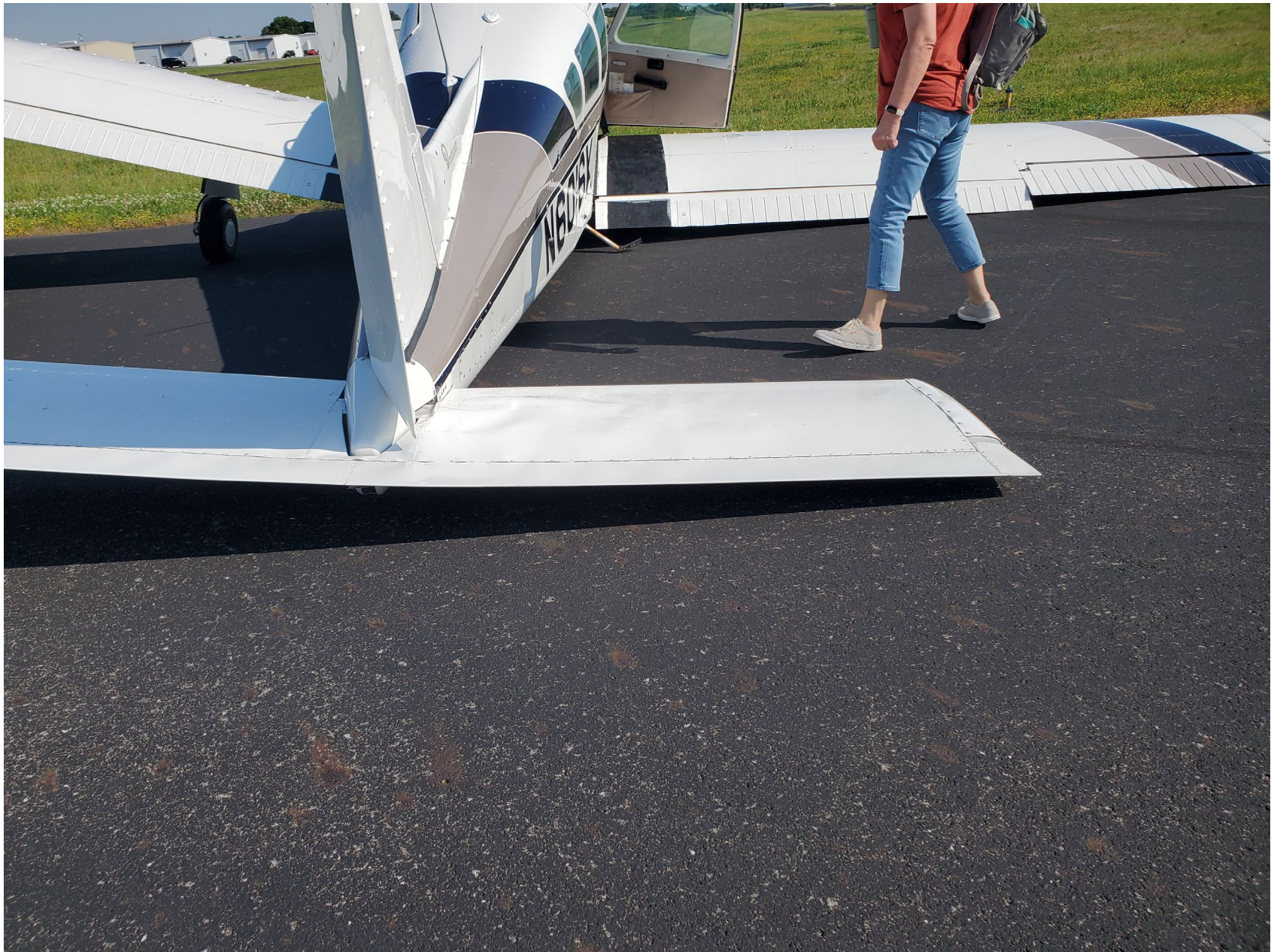
Photo 3 - Digital Photograph From Pilot. Aft View of the Airplane Where it Came to Rest. Note the Compression Wrinkle on the Upper Skin of the Right Side of the Stabilator.
