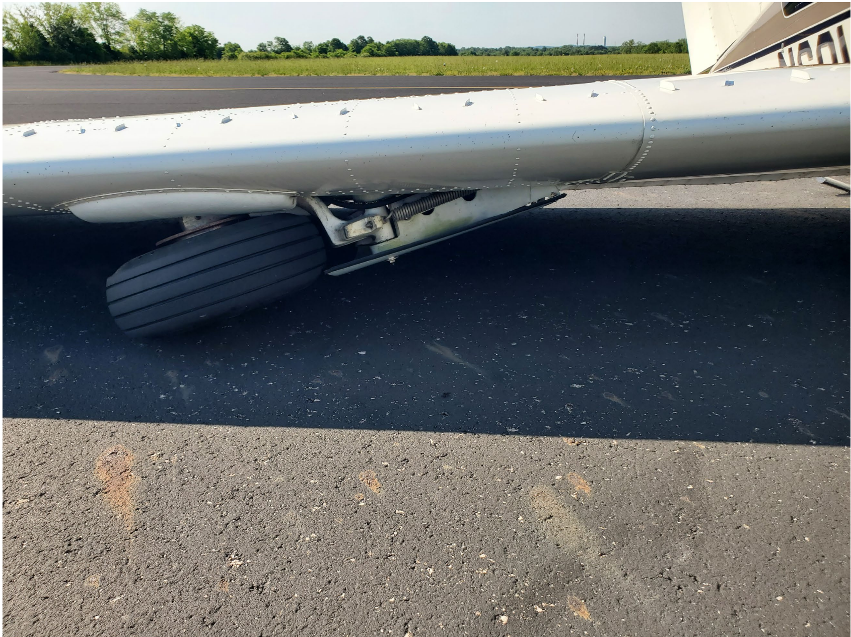
Photo 2 - Digital Photograph From Pilot. View of the Collapsed Right Main Landing Gear.
