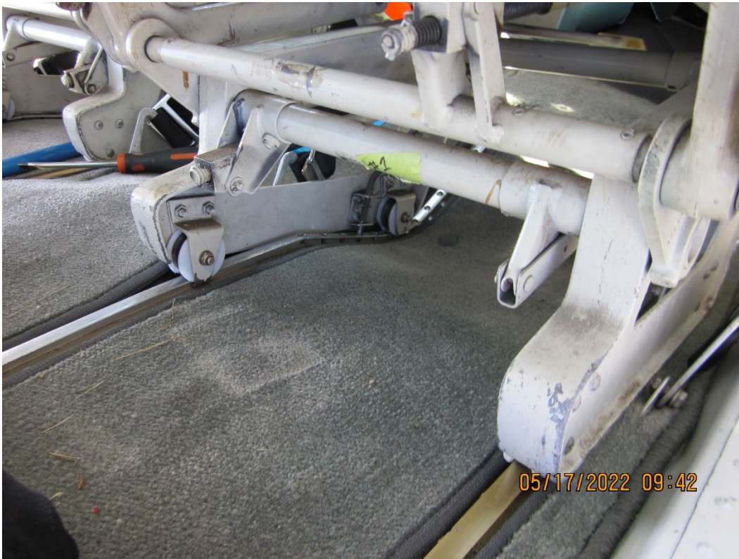
Photograph 5 – Accident airplane, buckled floorboards under forward right seat.
