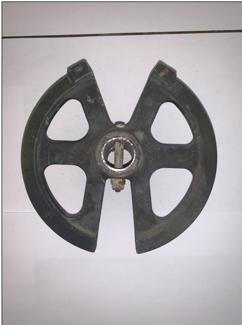
Figure 11: Overview of the elevator bellcrank.
