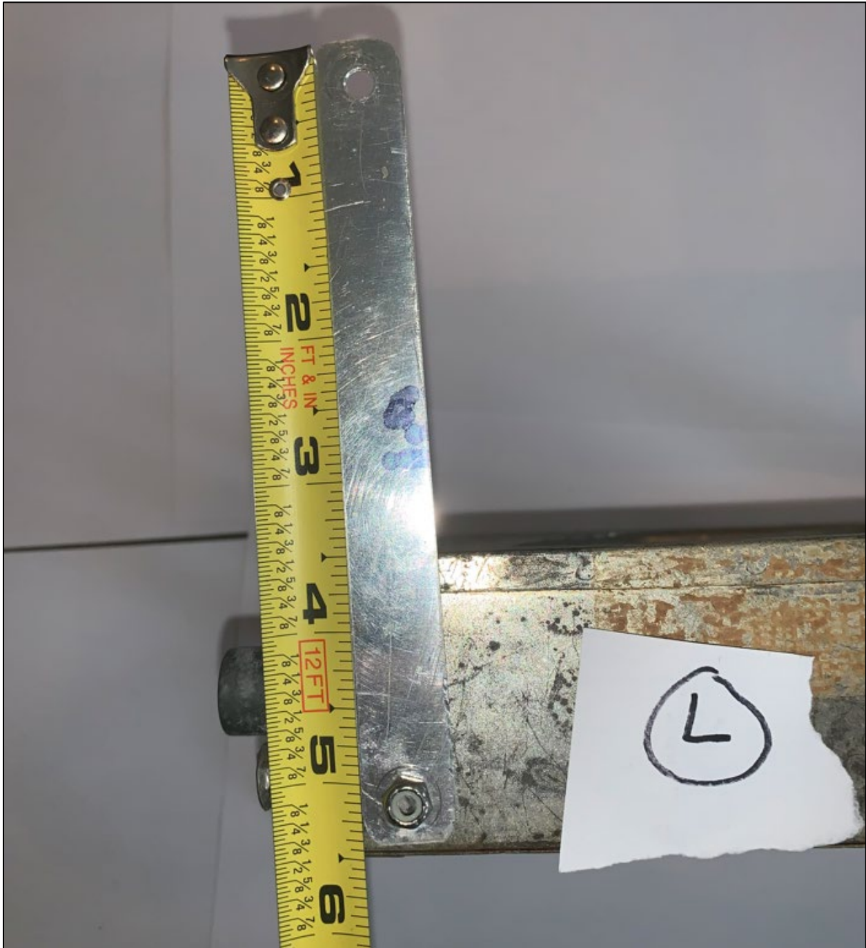
Figure 4: The metal strap on the KX-155 avionics tray measured about 5.5 inches in total length.
