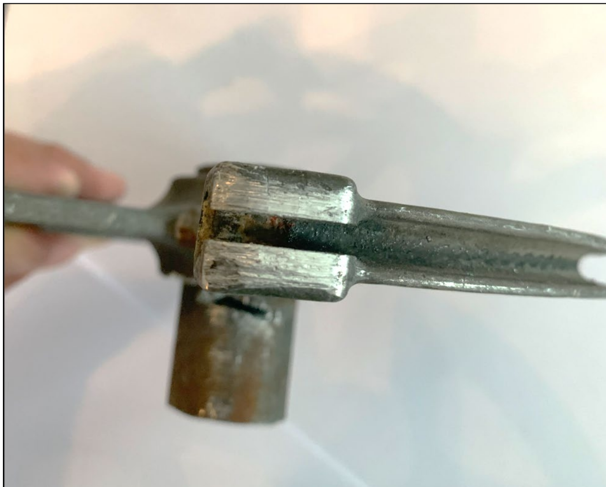
Figure 8: View of metal scraping and polishing as found on the elevator bell crank.
