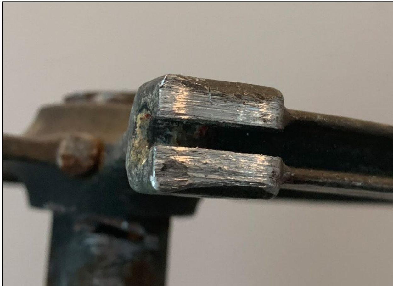
Figure 9: Additional view of metal scraping and polishing as found on the elevator bell crank.
