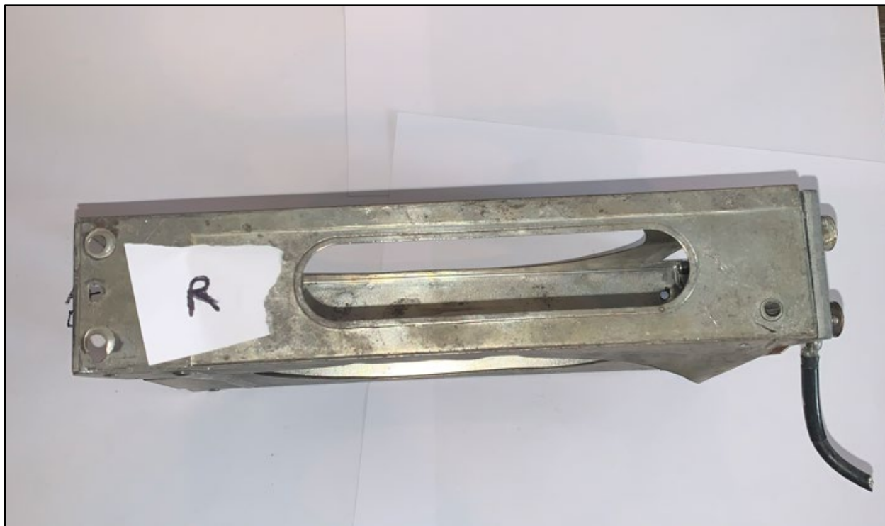
Figure 5: View of the right side of the KX-155 avionics tray. The right side did not possess a metal strap.
