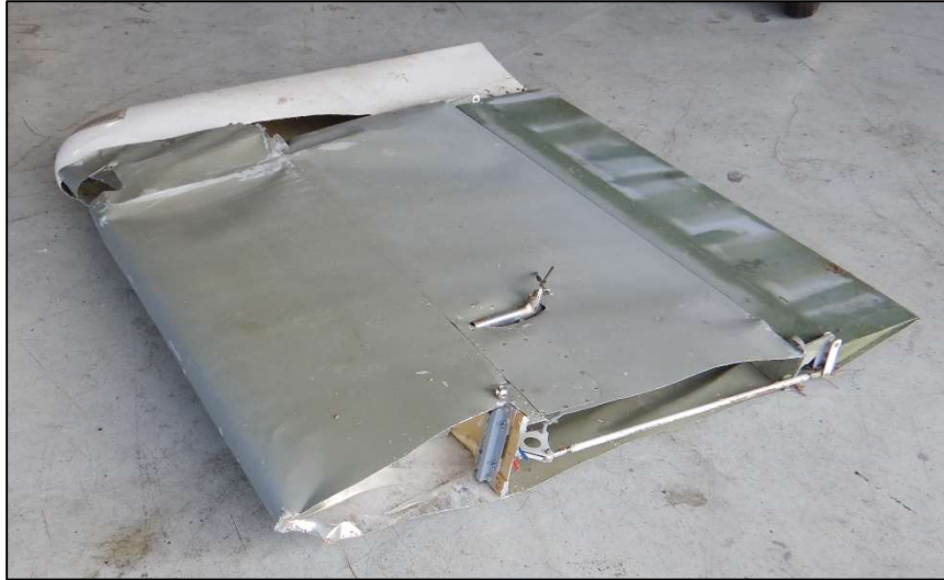
Photo 4 - Outboard section of left wing with aileron attached
