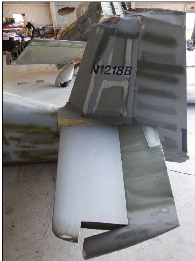
Photo 5 - Empennage with elevators and rudder intact
