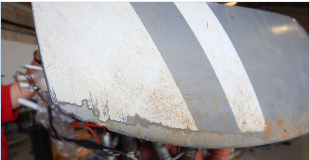
Photo 16 - Close-up view of leading edge gouging on blade 1
