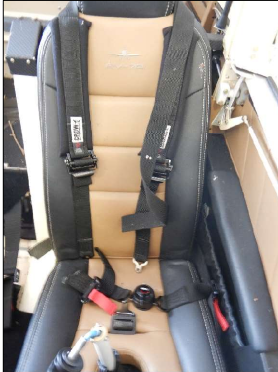
Photo 6 - Left pilot seat with lap belts attached to locking mechanism
