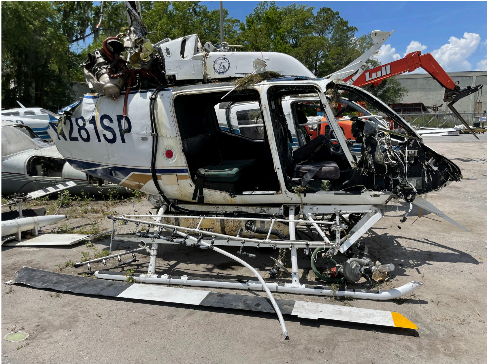
Photo 1 – Digital Photograph From Recovery Company. Right Side View of the Helicopter Following Recovery. Note the Separated Tailboom and Displaced Engine.
