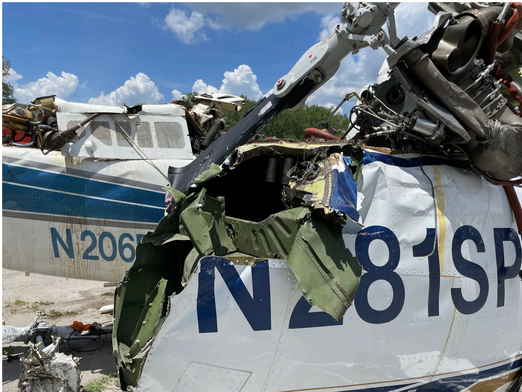
Photo 2 - Digital Photograph From Recovery Company. Right Side View of the Helicopter Following Recovery. Note the Structural Damage, Separated Tailboom, and Displaced Main Rotor Assembly.
