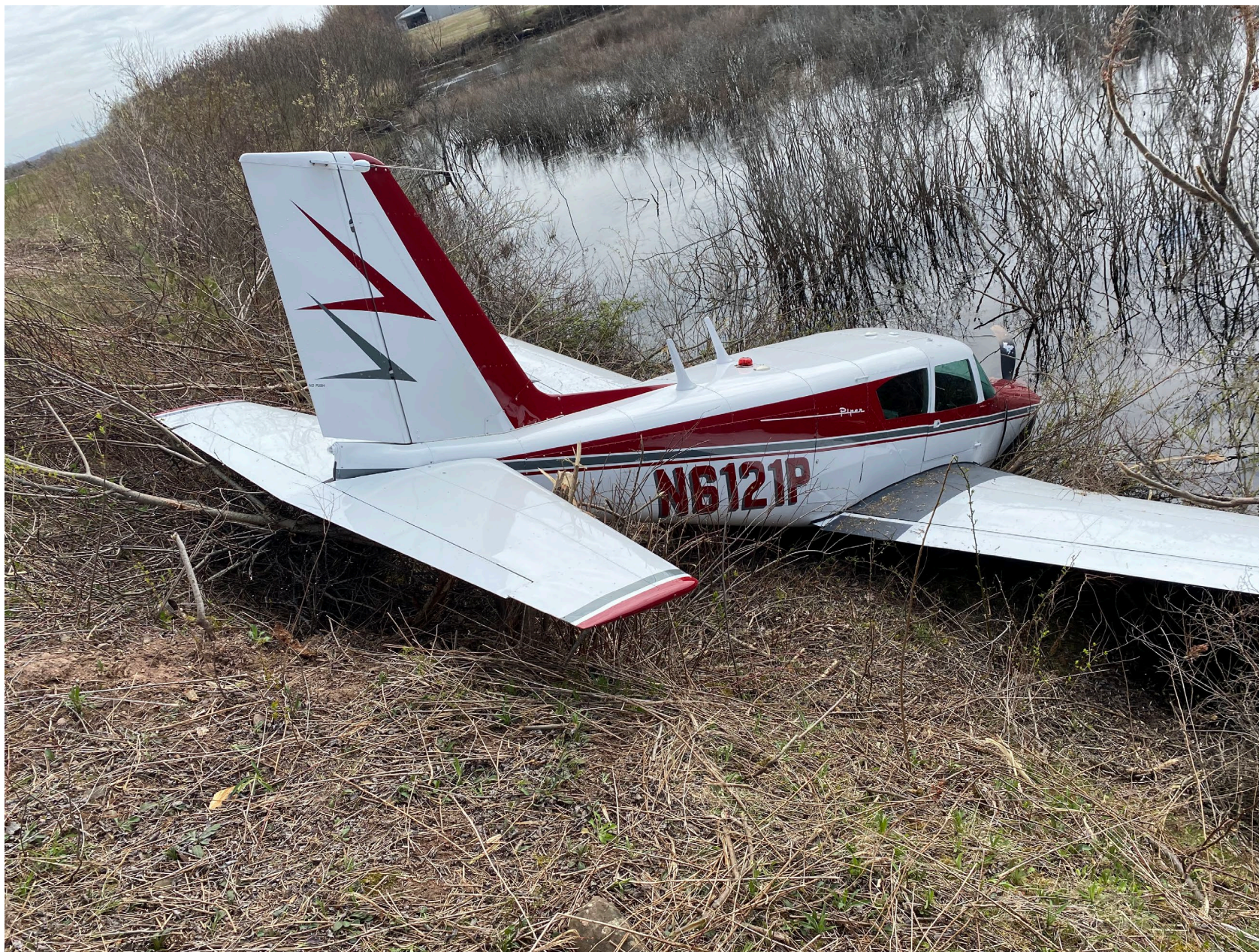
Photo 2 - FAA Digital Photograph. Right Rear Quartering View of the Airplane Where it Came to Rest down the Embankment. Not Visible are the outer Portion of the right wing, Upper Part of the Vertical Stabilizer and Rudder, and Outer Portion of the Left Wing.
