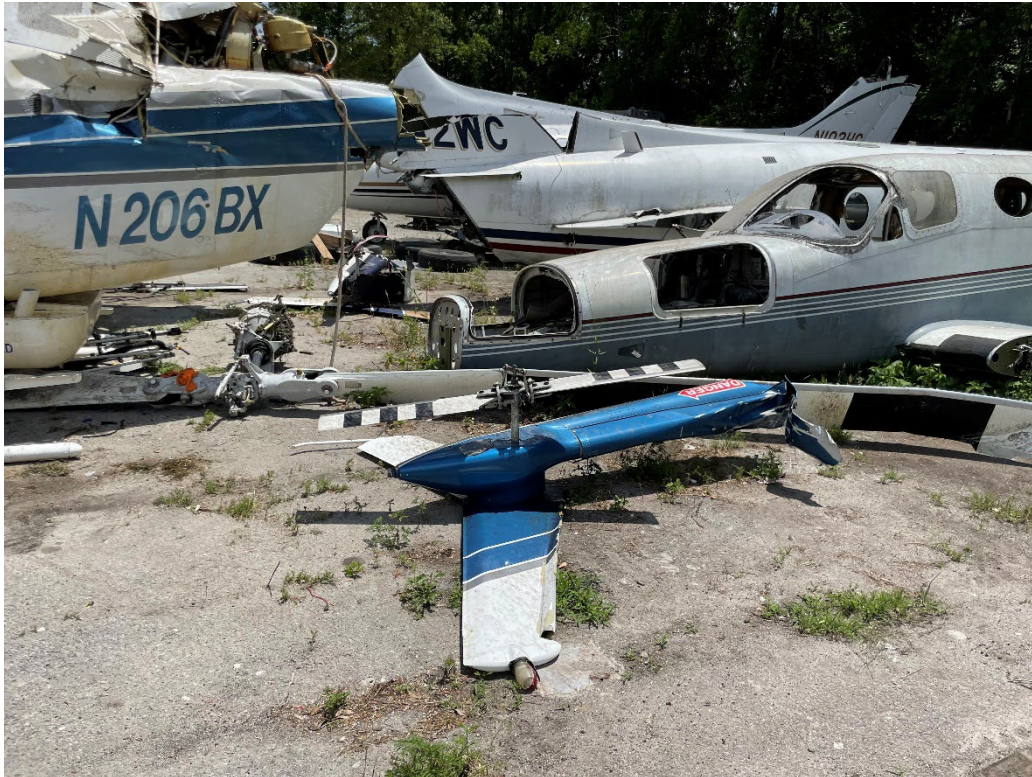
Photograph 4 – Accident Helicopter – Separated tailrotor.
