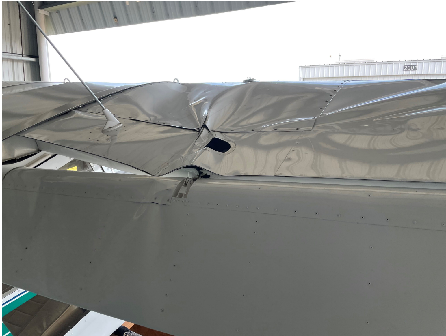
Photo 6: Overview of the right wing damage, inboard trailing edge (FAA Photo)
