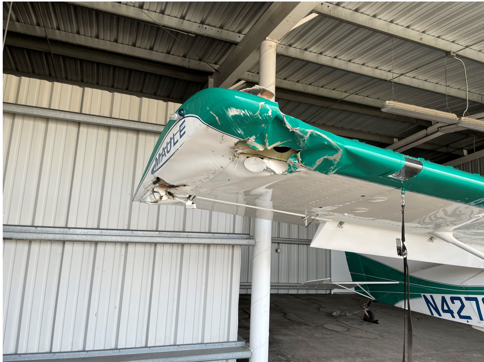
Photo 3: Airplane's right wing tip damage (FAA Photo)
