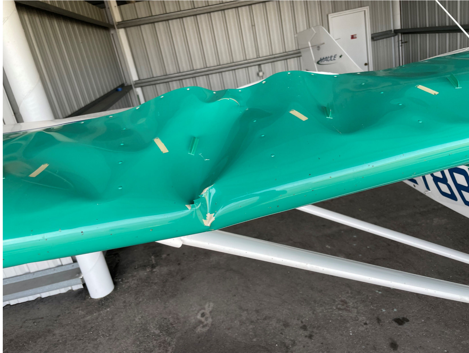
Photo 4: Overview of the right wing damage, leading edge (FAA Photo)
