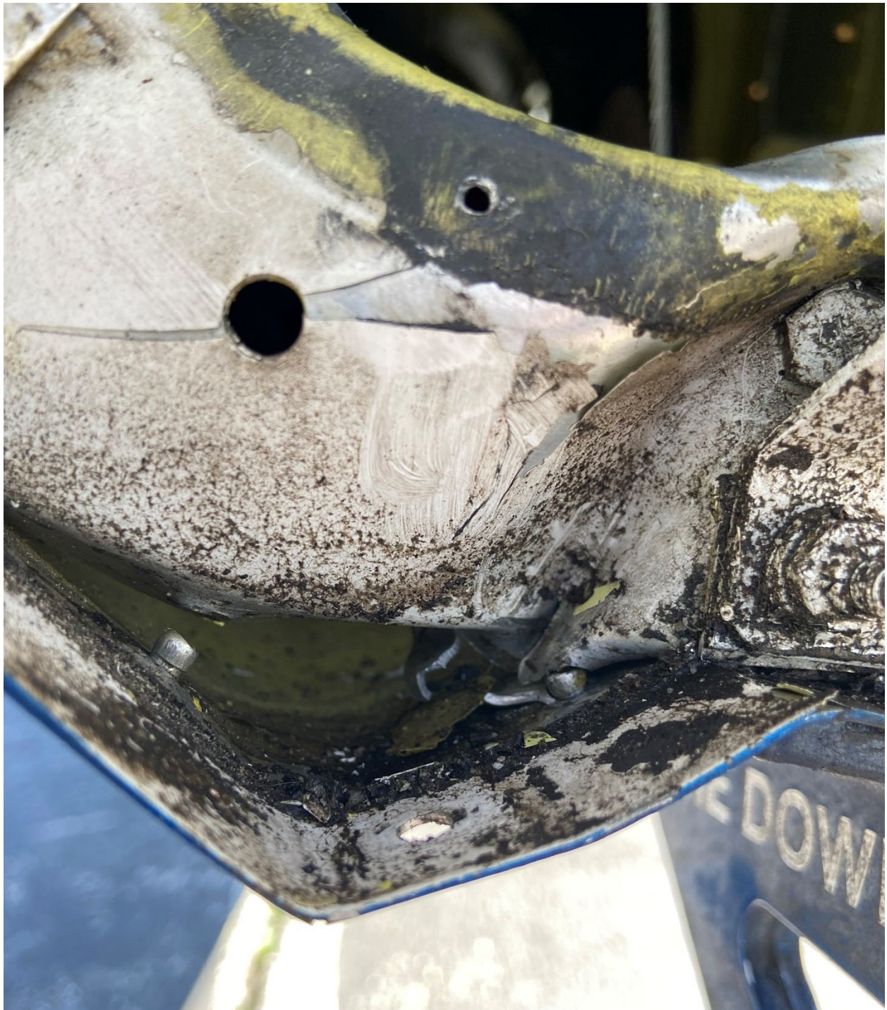
Photograph 2 – Close-up of damage to accident airplane tail section.
