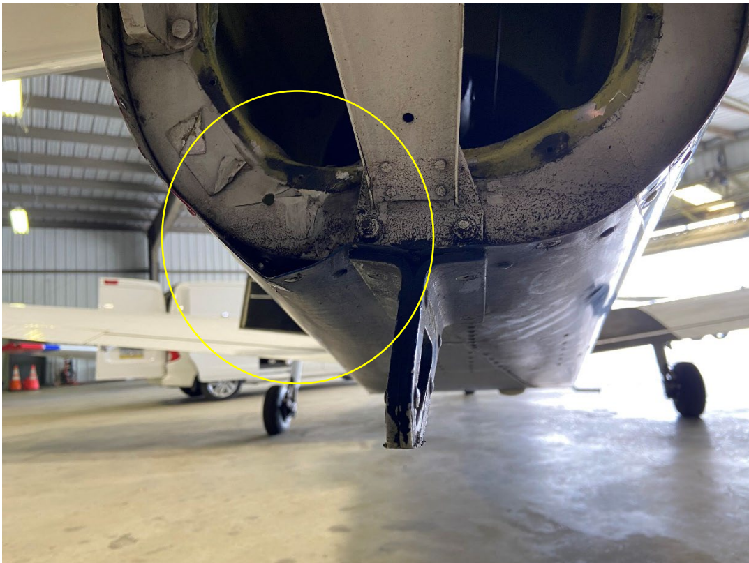
Photograph 1 – Accident airplane damage to tail section and tie down.
