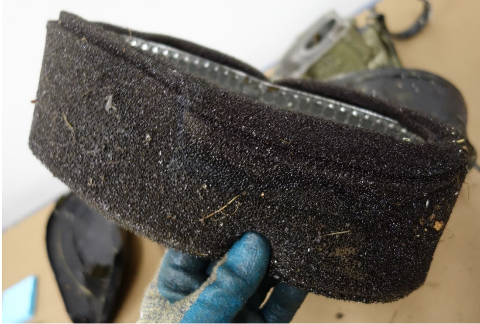
Figure 12. View of air inlet filter.
