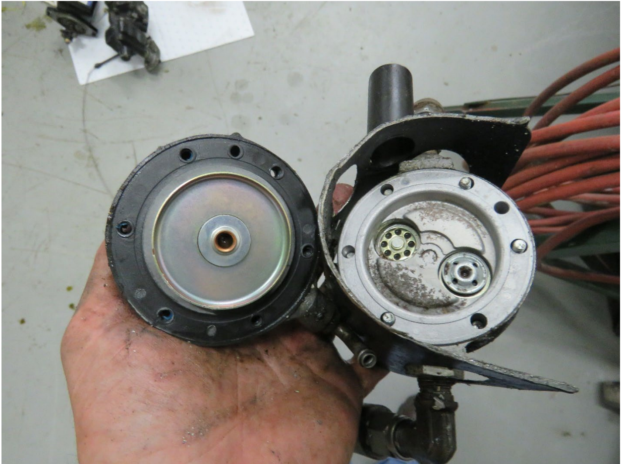
Figure 10. View of disassembled fuel pump.
