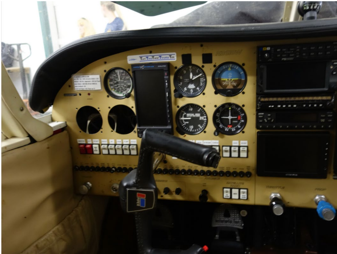
Figure 3. Photograph of accident airplane cockpit. Note no placard on the left side wall.
