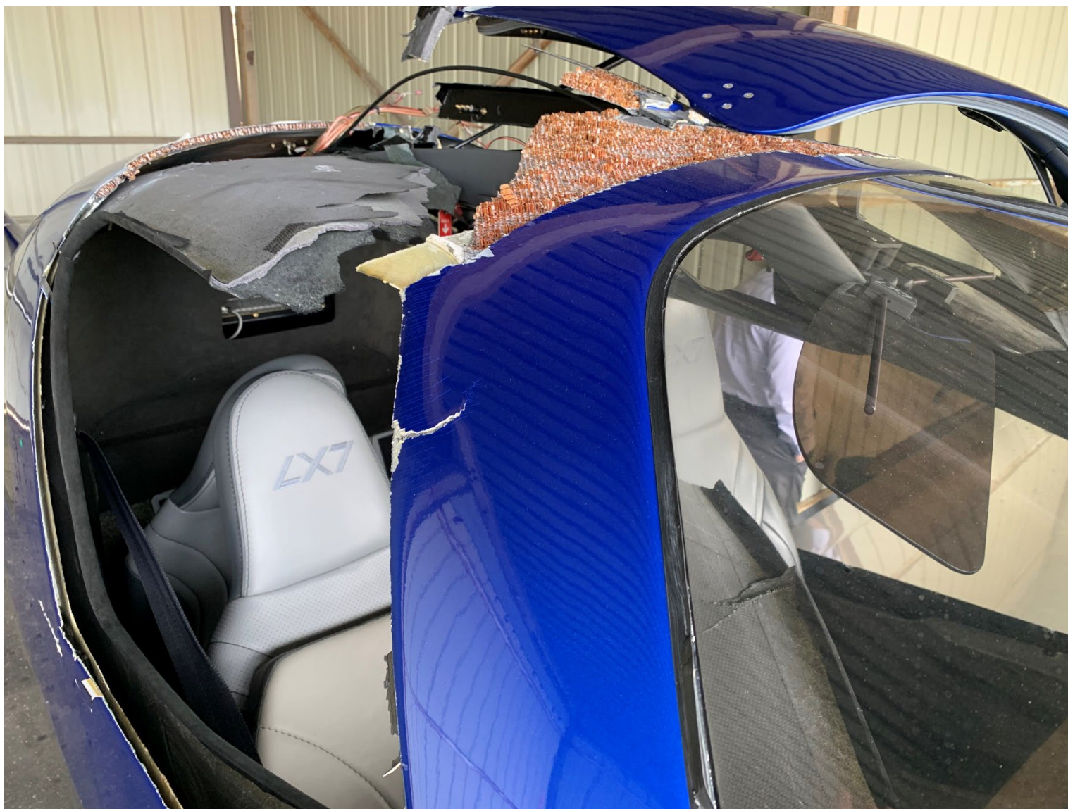
Photograph 1 - View of right window and roof missing. (Courtesy of FAA)
