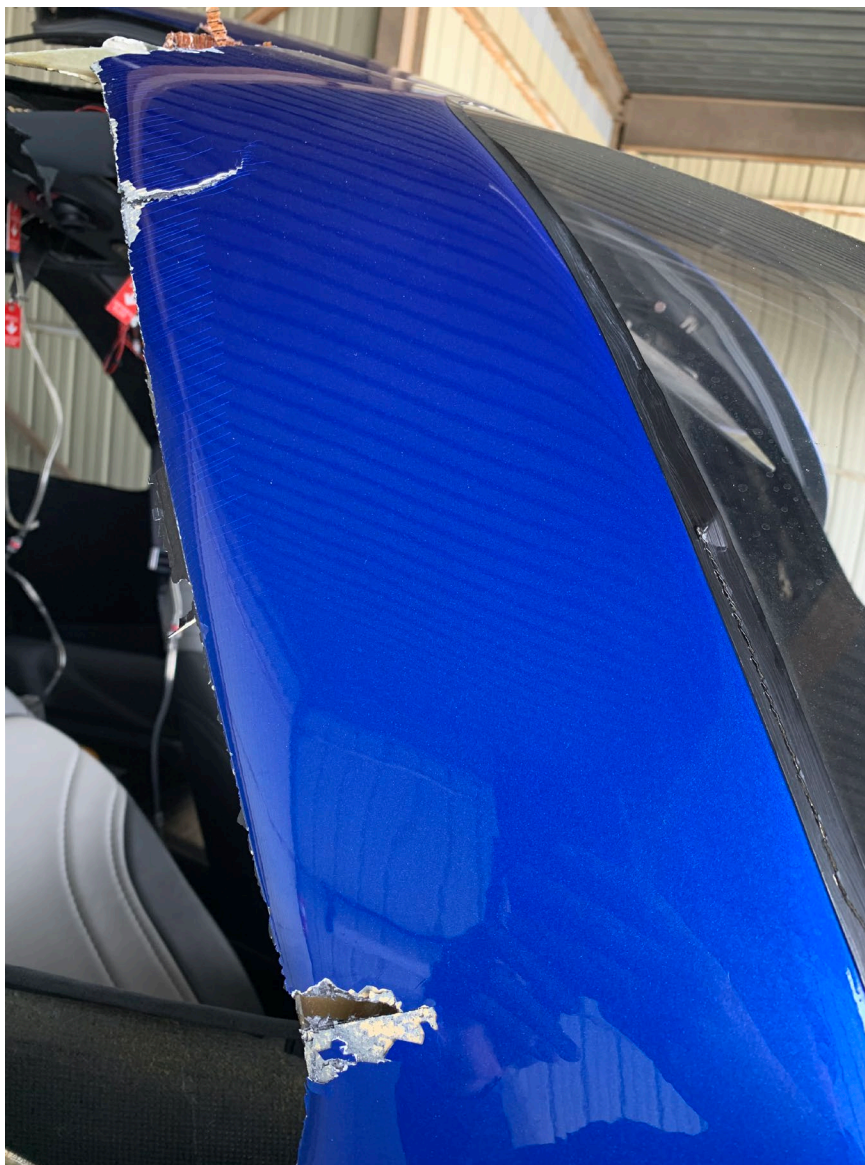
Photograph 3 - View of damage along forward edge of window. (Courtesy of FAA)
