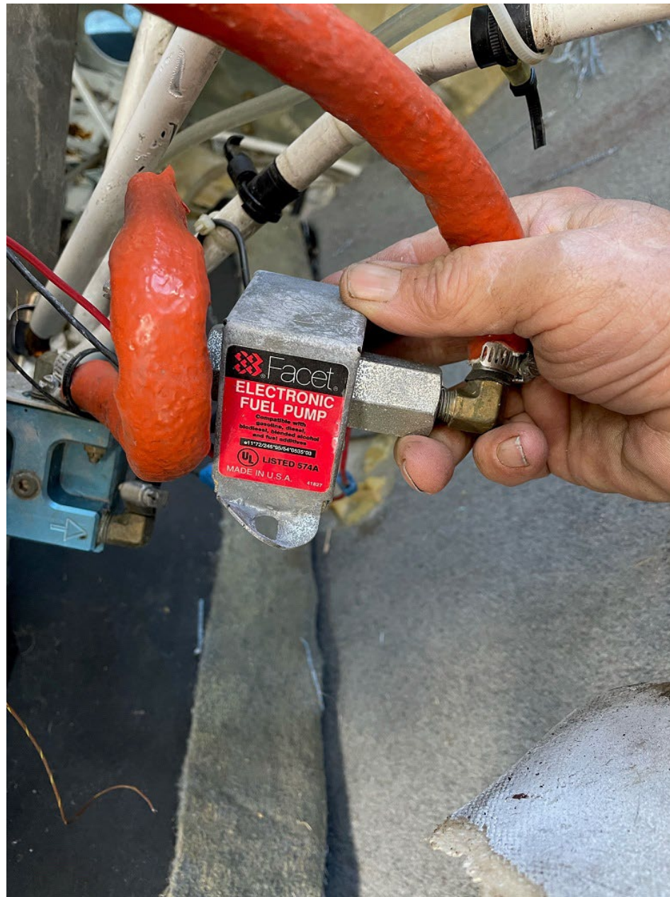
Photo 6 – Electric Boost Pump (Photo Courtesy of Airport Manager)
