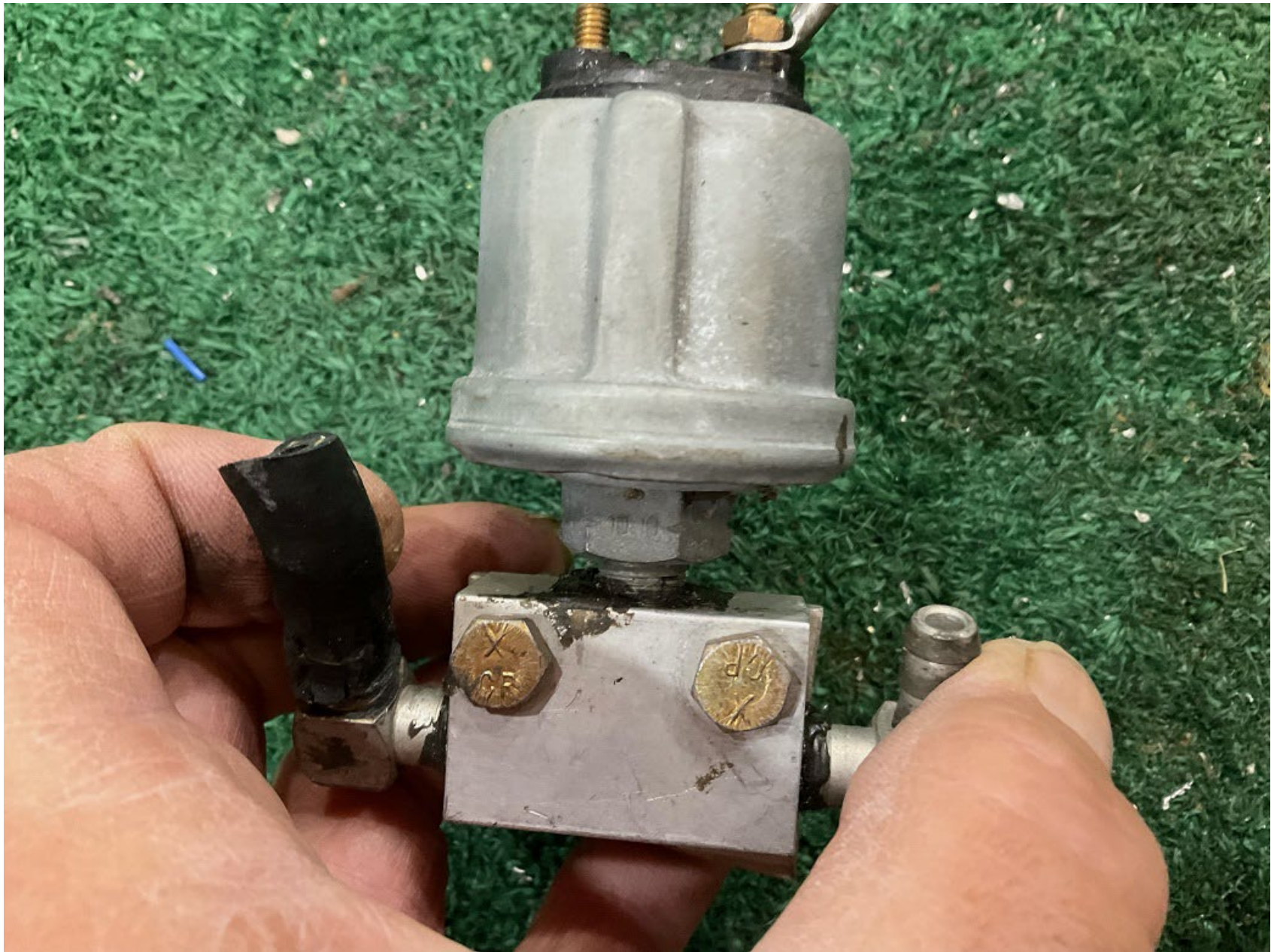
Photo 5 – Fuel Pressure Sensor (Photo Courtesy of Airport Manager)
