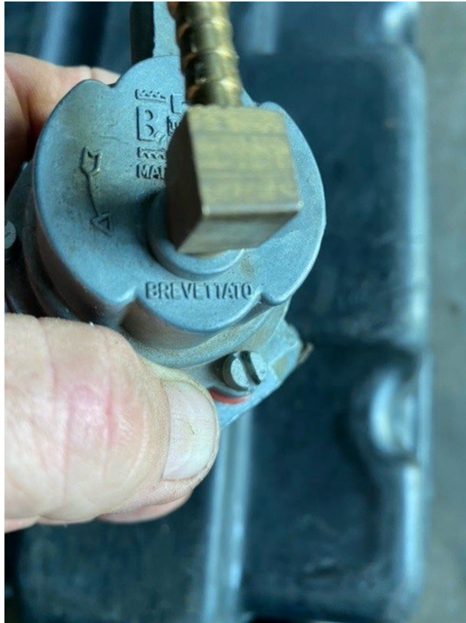
Photo 3 – Engine Driven Fuel Pump (Photo Courtesy of Airport Manager)
