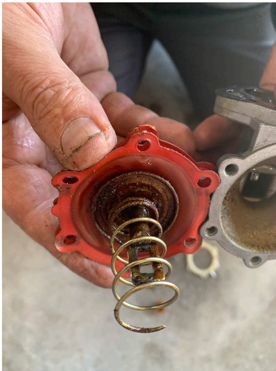
Photo 4 – Engine Driven Fuel Pump Diaphragm Return Spring (Photo Courtesy of Airport Manager)
