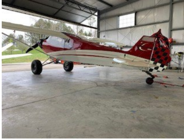
Photograph 3 – Accident Airplane – Damaged rudder.
