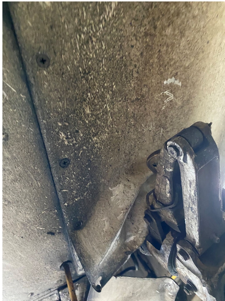
Photo 5: View of the fuselage damage near the nose landing gear (Photo Courtesy of FAA)
