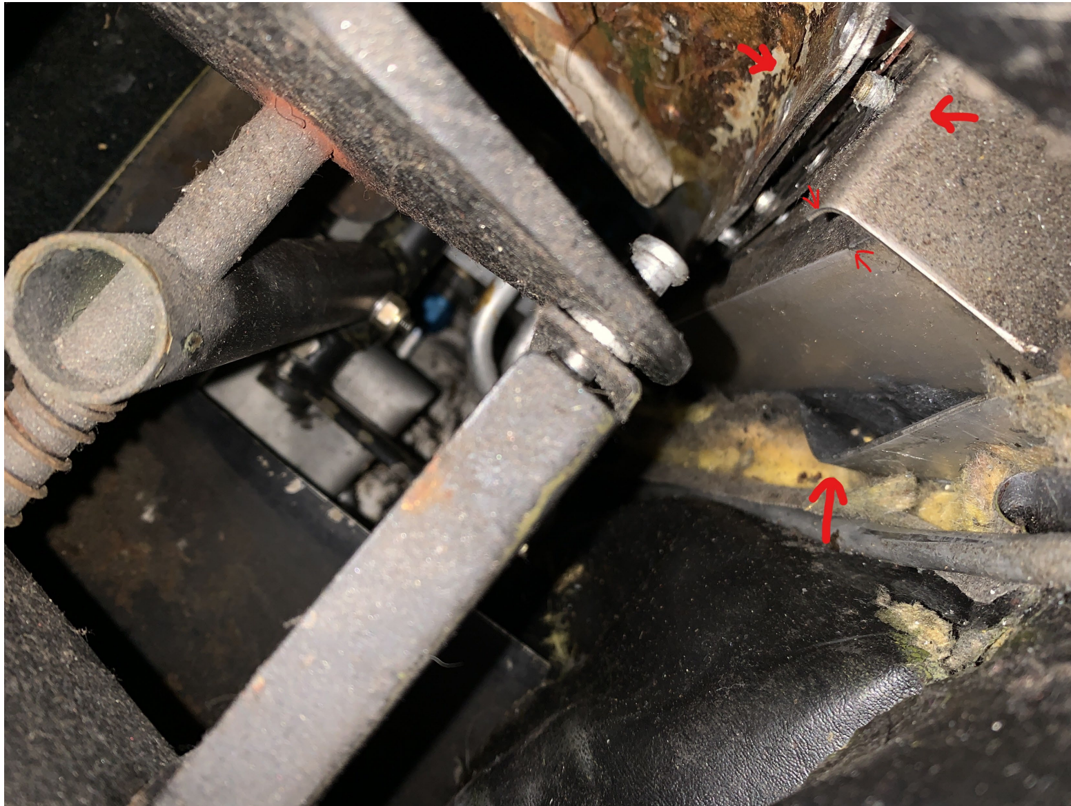
Photo 3: View of the fuselage damage near the rudder pedals (Photo Courtesy of FAA)
