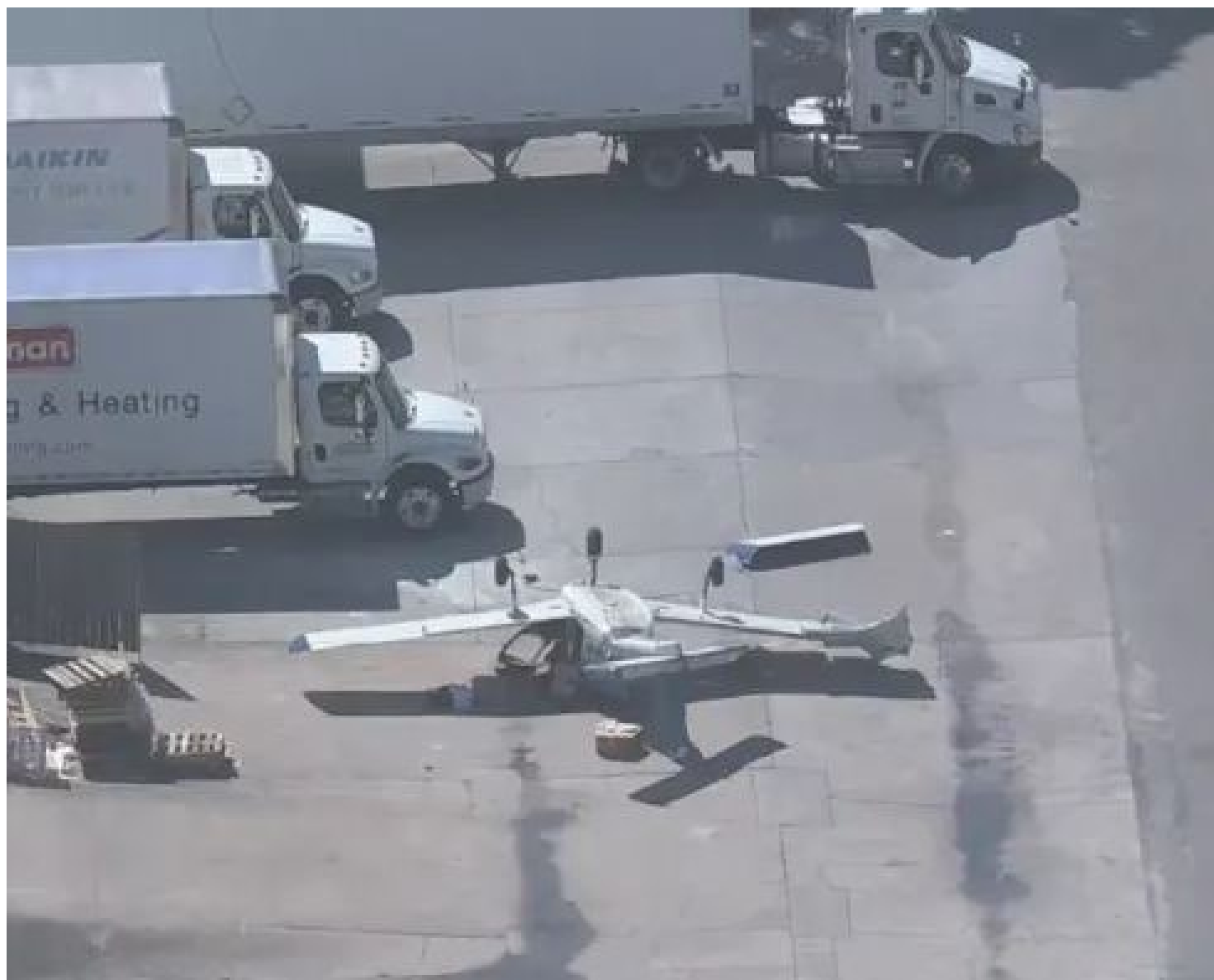
Photo 1 – main wreckage, inverted (FAA)
