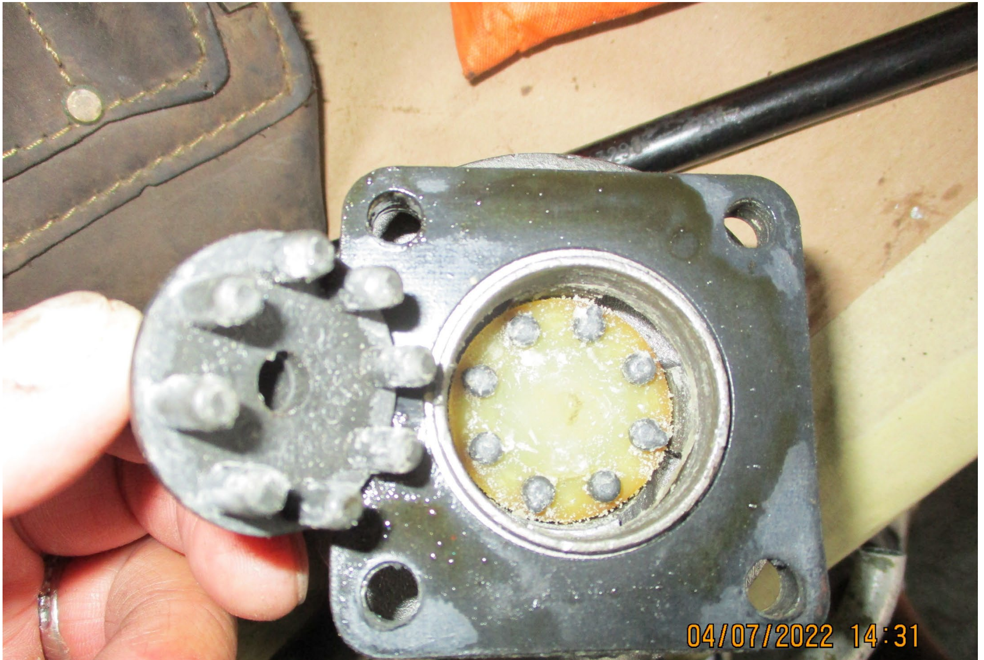
Photo 7 – vacuum pump, coupling destroyed
