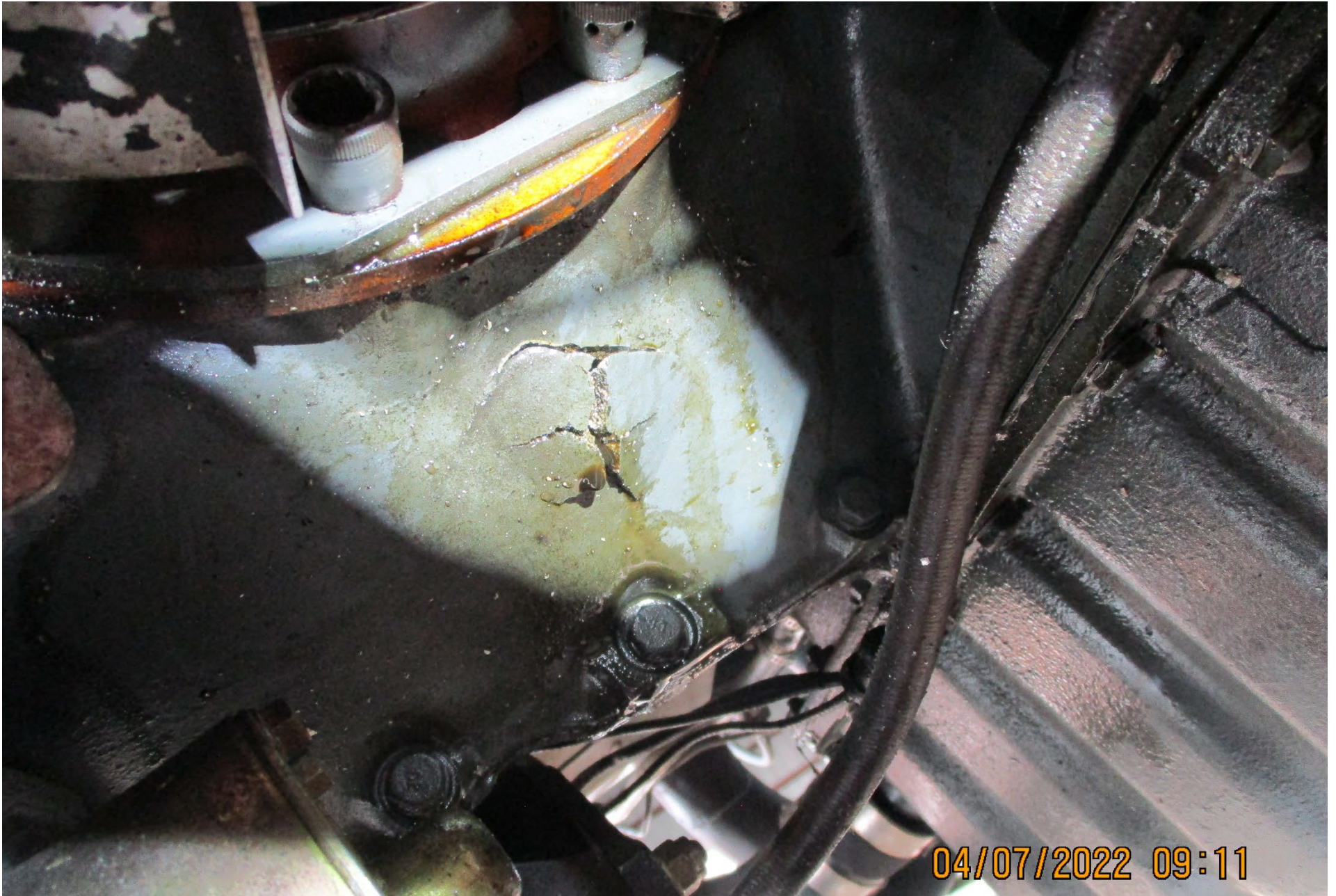
Photo 3 – case fractured from inside
