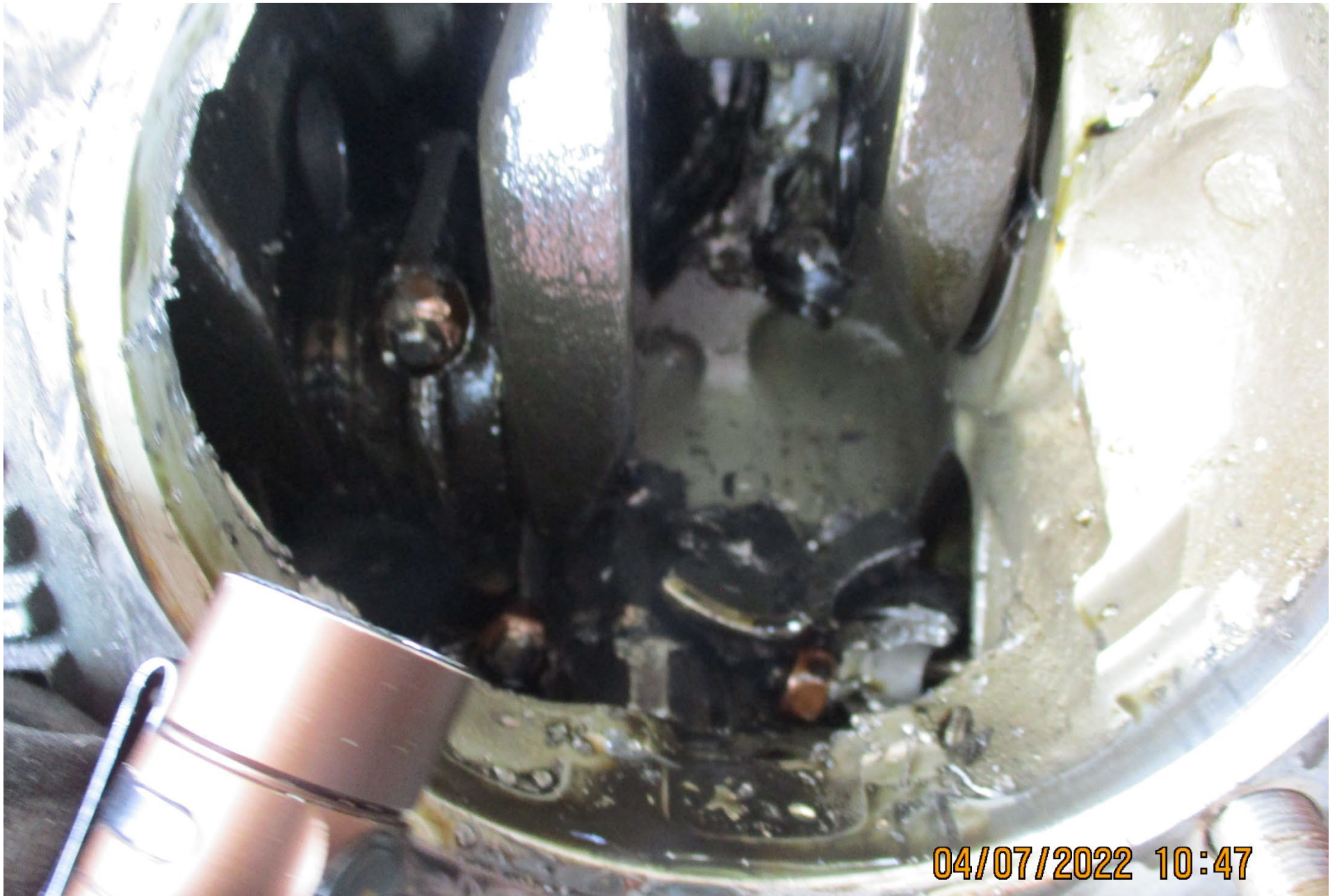
Photo 4 – metal parts at bottom of case half
