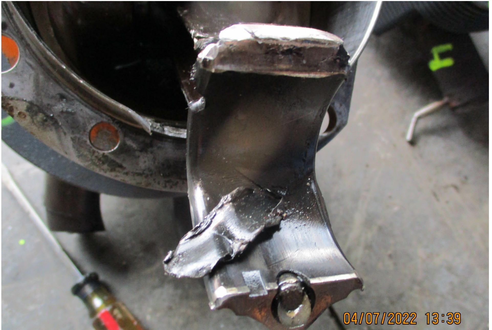
Photo 5 – piston rod, fractured with bearing destroyed
