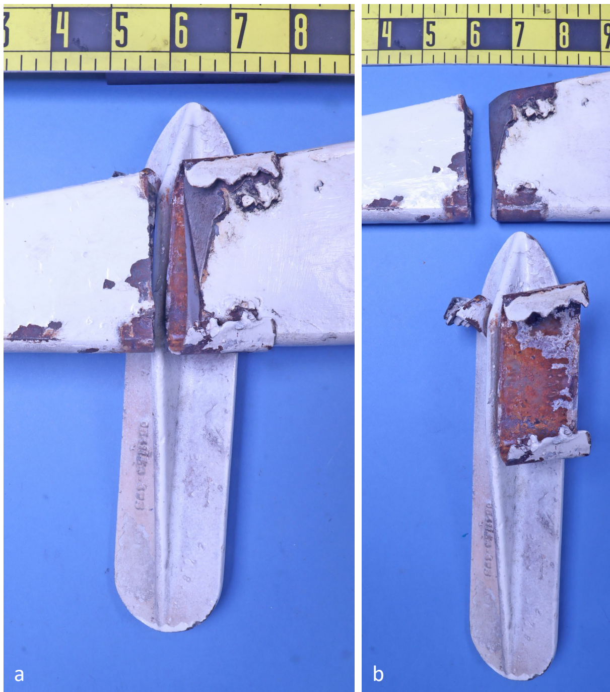
Figure 4. View a shows an image of the upper and lower portions of the fractured spring strut with the step and bracket positioned in its approximate pre-accident location. Tack welds between the step bracket and the bottom face of the spring strut are noted. In view b, the underside of the bracket exhibits corrosion product, loose scale, and paint stains from wicking paint
