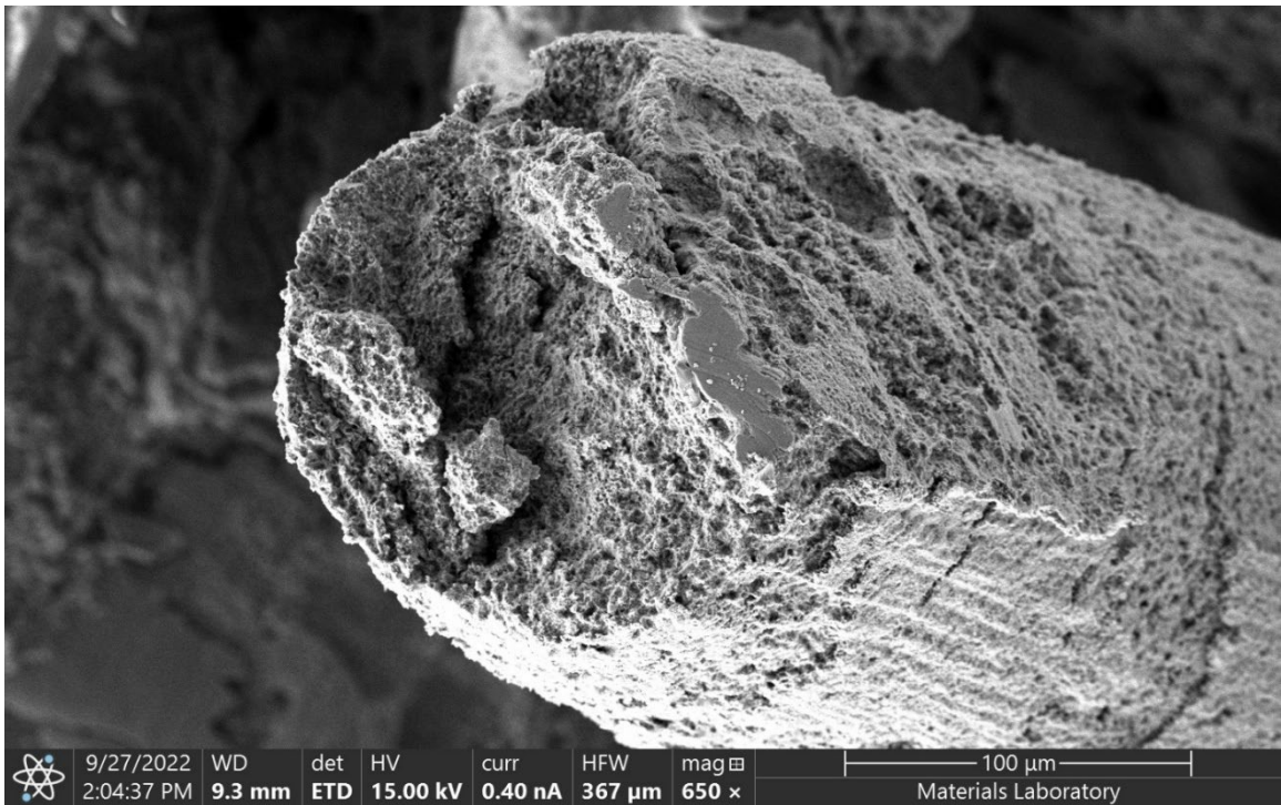
Figure 16. SE micrograph of cup-shaped wire fracture surface.
