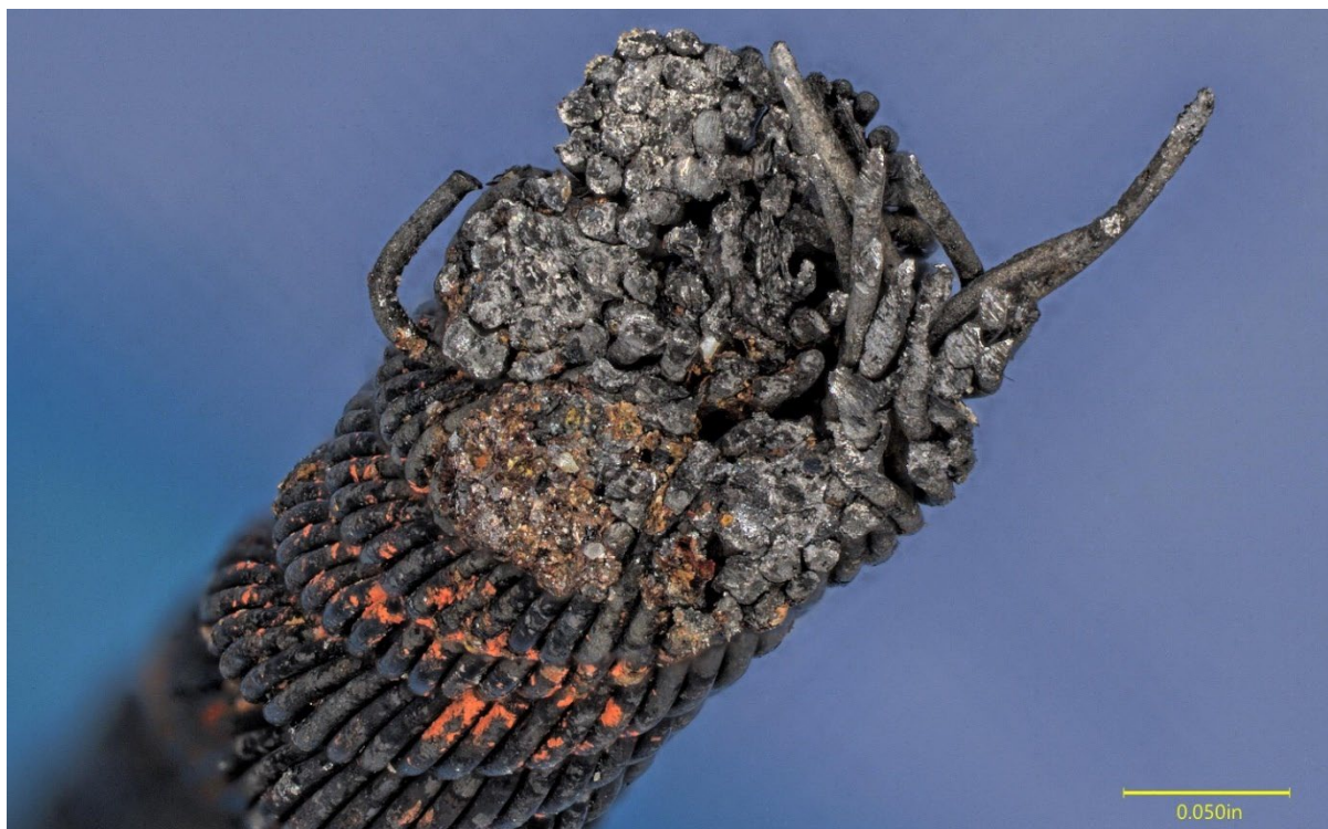
Figure 8. View of the left side cable remnant fracture surface, after first cleaning.
