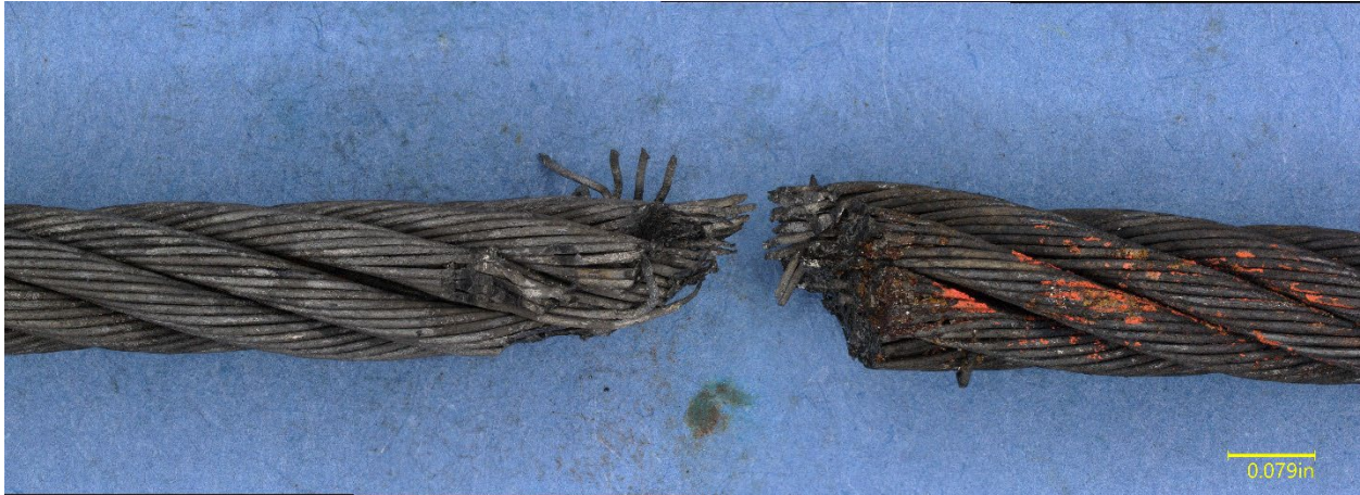
Figure 5. View of the fractured ends of the aileron cable, positioned in the location consistent at fracture, post-cleaning of both sides.
