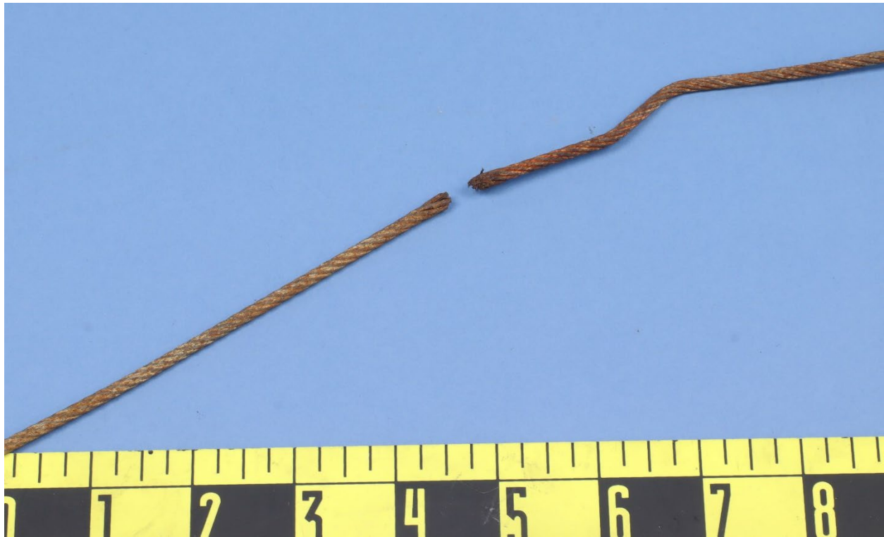
Figure 2. Closer view of the fractured region of the aileron cable.
