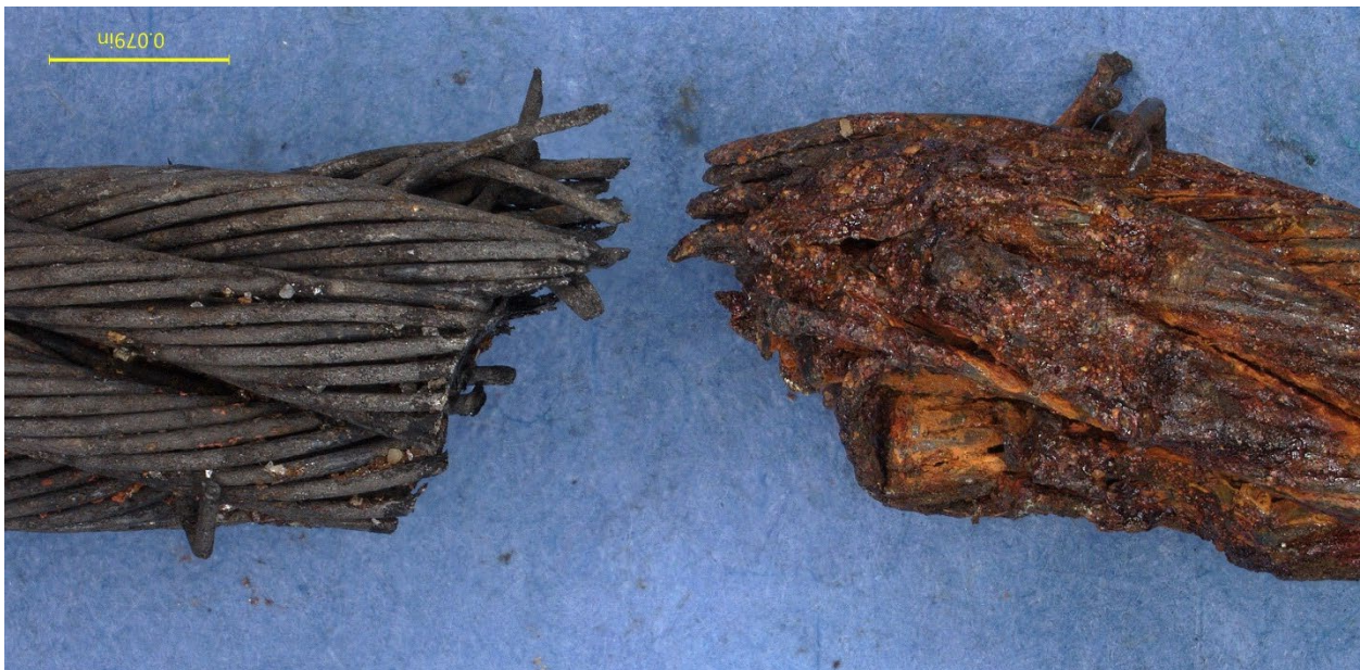
Figure 4. The fractured ends of the left cable remnant (left side, post-cleaning) and the right cable remnant (right side, as-received).
