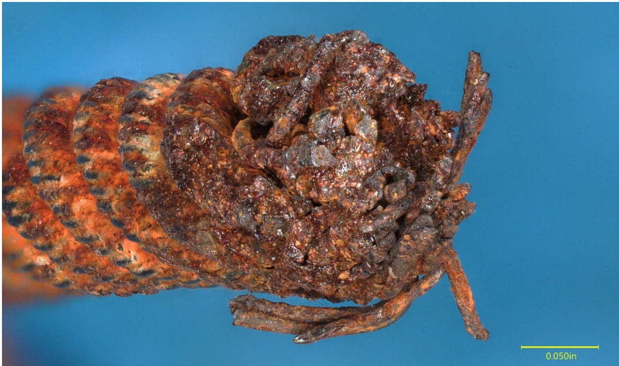
Figure 6. View of the right side cable remnant fracture surface, as received.
