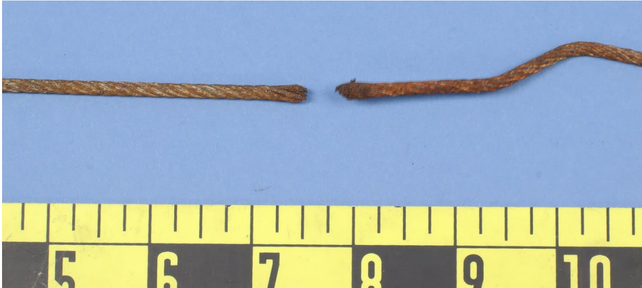
Figure 3. View of the fractured aileron cable ends, positioned to face each other, as received.
