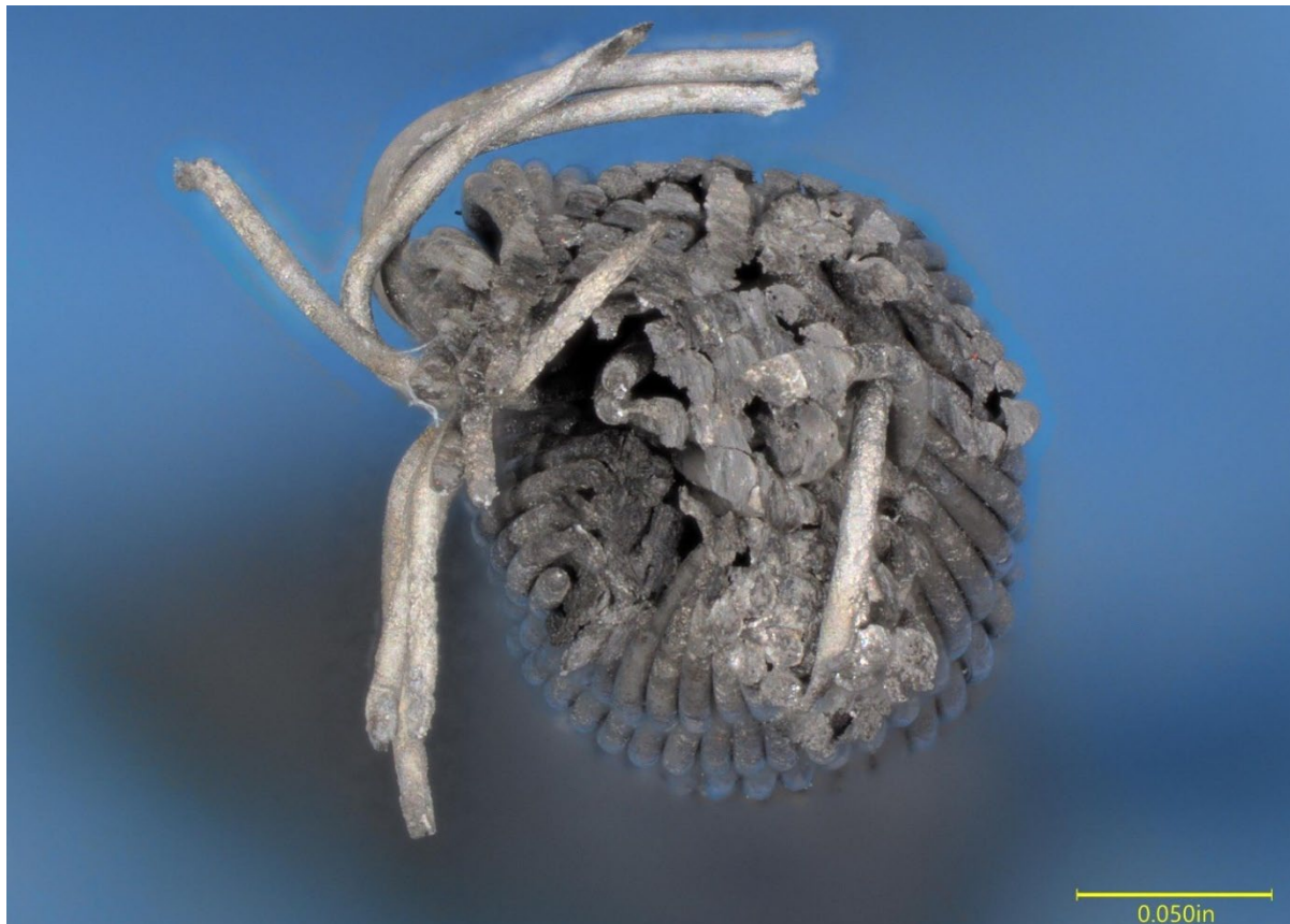
Figure 7. View of the right side cable remnant fracture surface, after cleaning.
