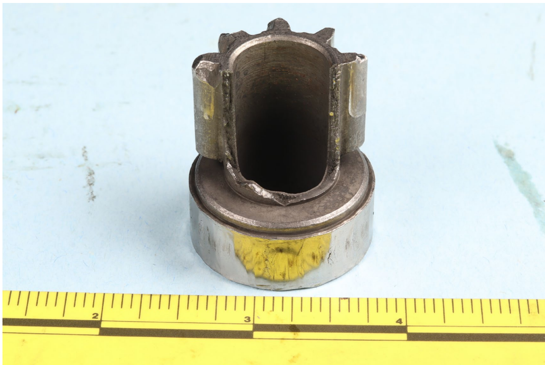
Figure 6. Pinion gear with missing portion of gear teeth and overstress fracture.
