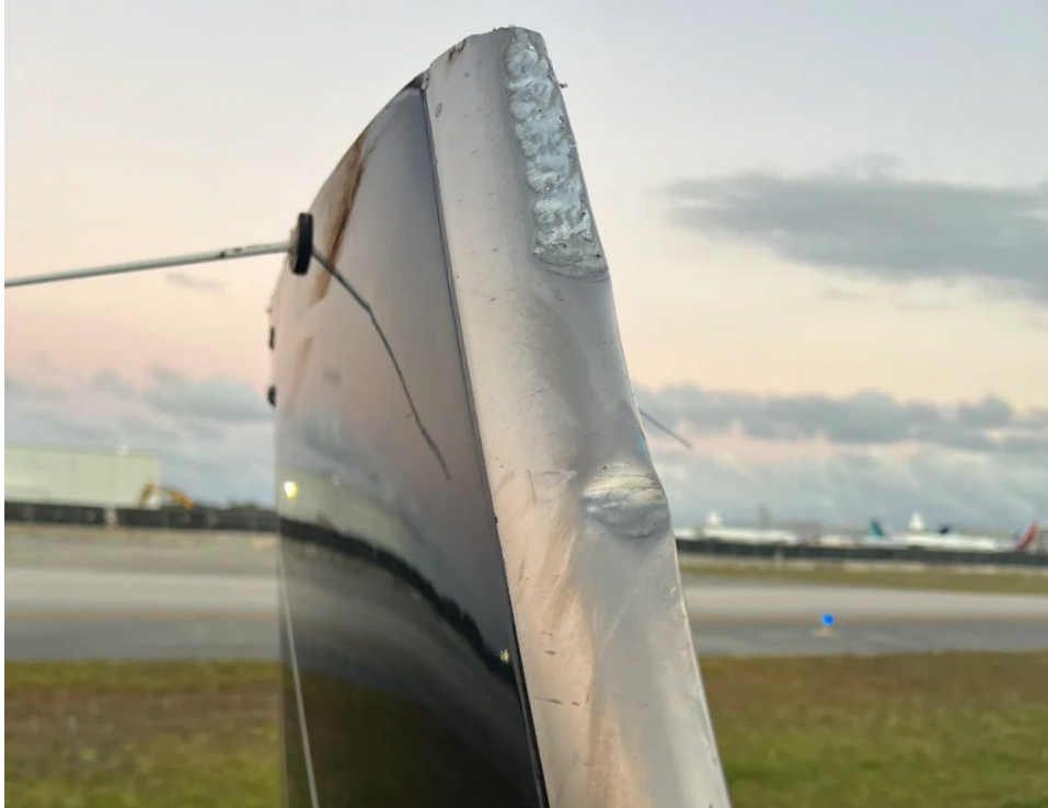
Photograph 2 – SR-22 vertical stabilizer damage.
