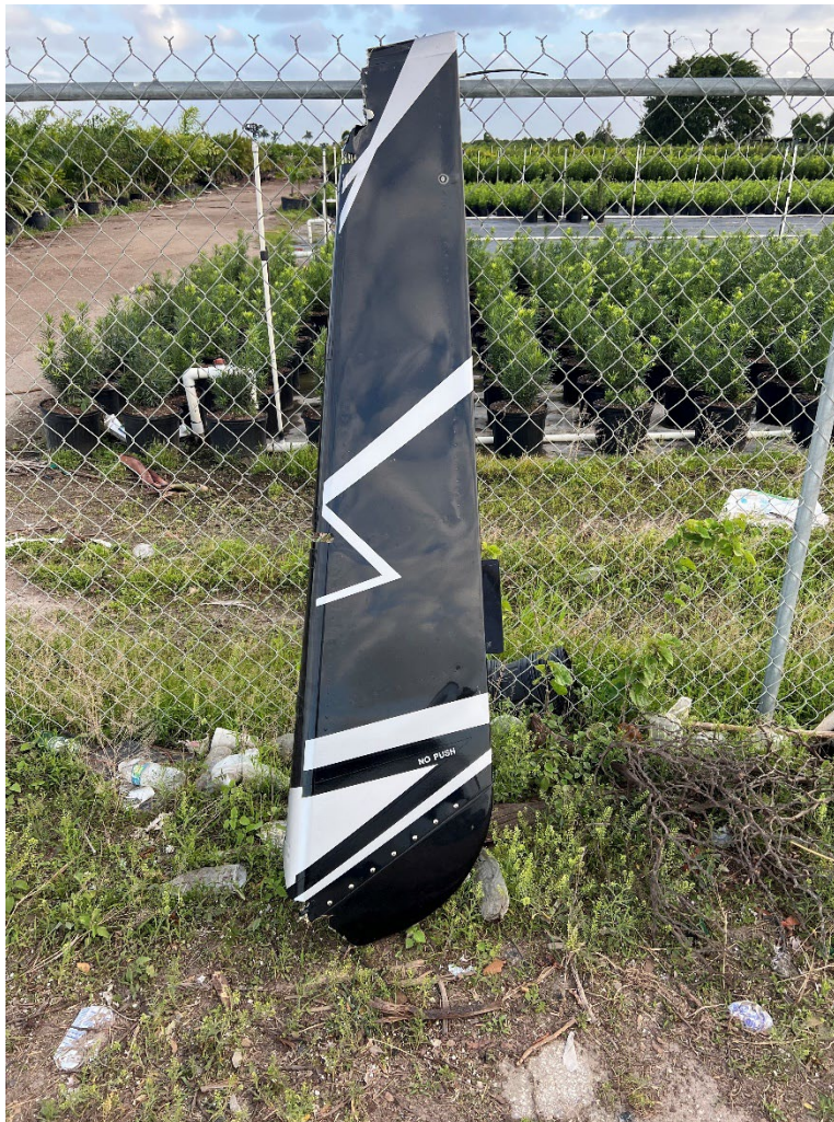
Photograph 1 – SR-22 separated rudder.
