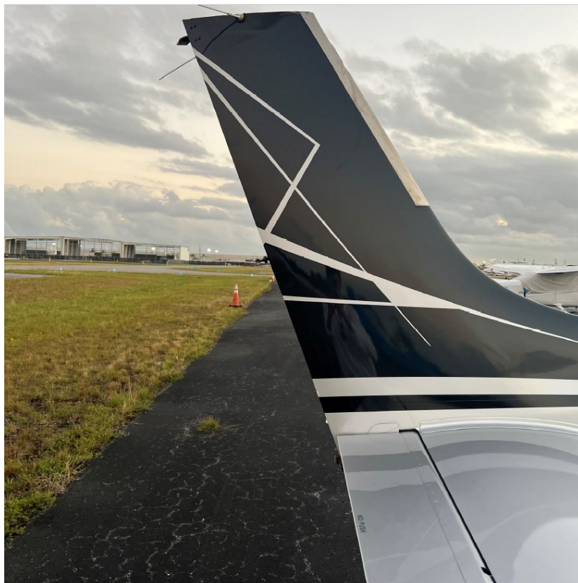
Photograph 3 – SR-22 vertical stabilizer with missing rudder.
